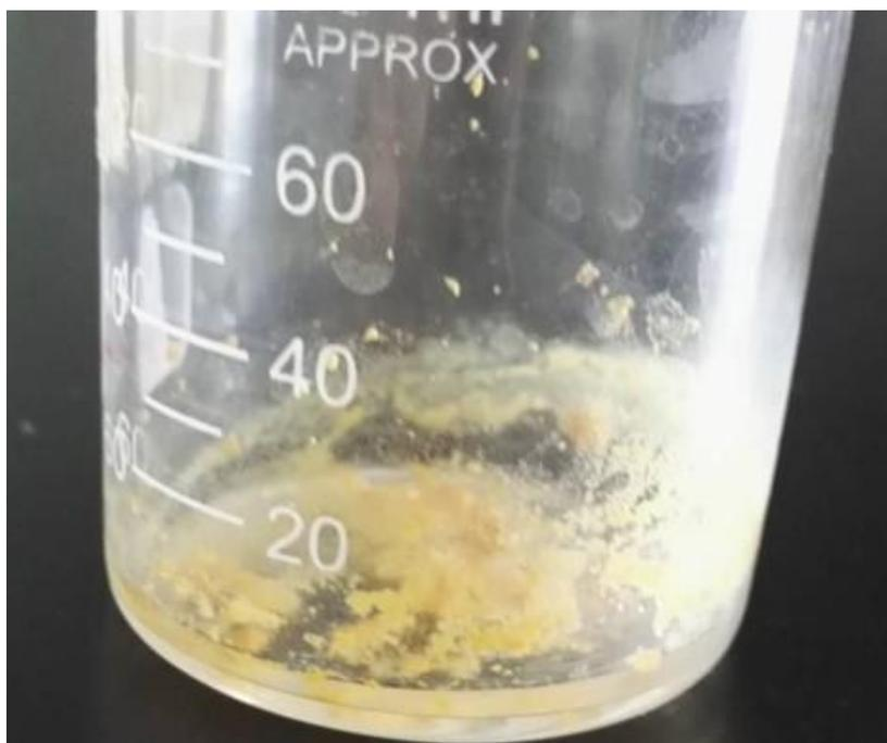
Figure S2. The organics recovered from spent catalysts by distillation.
