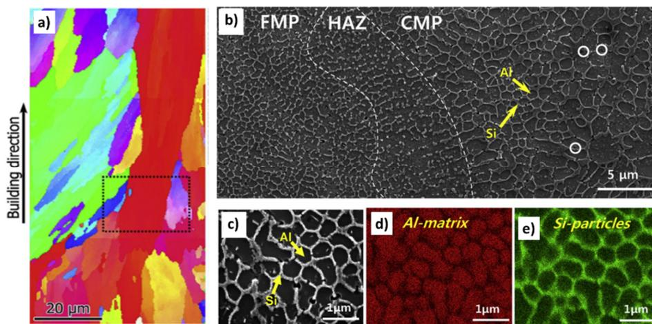
**Figure 2.** (a) Electron backscatter diffraction (EBSD) inverse pole figure (IPF), adapted from [31], with permission from © 2016 Elsevier, (b,c) SEM images and (d) Al- and (e) Si EDS maps of an as-built AlSi10Mg sample, adapted from [22], with permission from © 2016 Elsevier.
