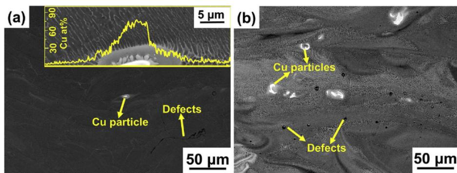
**Figure 4.** Backscattered Electrons (BSE) SEM micrographs of LPBF (a) Al-6Cu and (b) Al-40Cu alloy (inset: Cu distribution across the Cu-rich zone), adapted from [38], with permission from © 2018 Elsevier.
