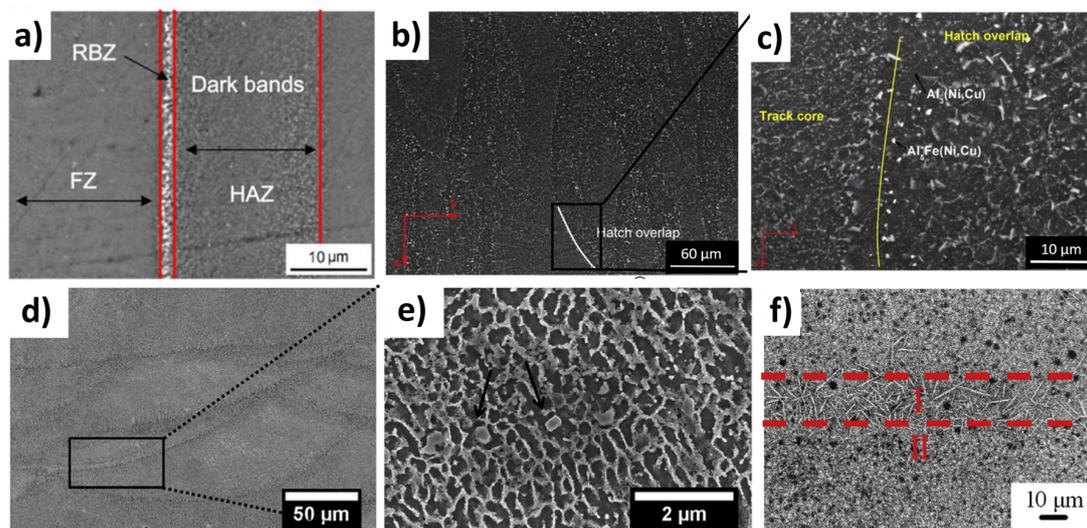
**Figure 9.** SEM images of (a) FVS0812, adapted from [82], with permission from © 2015 Cambridge University Press; (b,c) Al-Si-Ni-Fe water quenched and aged at 250 °C for 5 h, adapted from [83], with permission from © 2019 Elsevier; (d,e) Al-Si-Ni, adapted from [33], with permission from © 2017 Elsevier; and (f) Al-20Si-Fe-Cu-Mg adapted from [68], with permission from © 2016 Elsevier.
