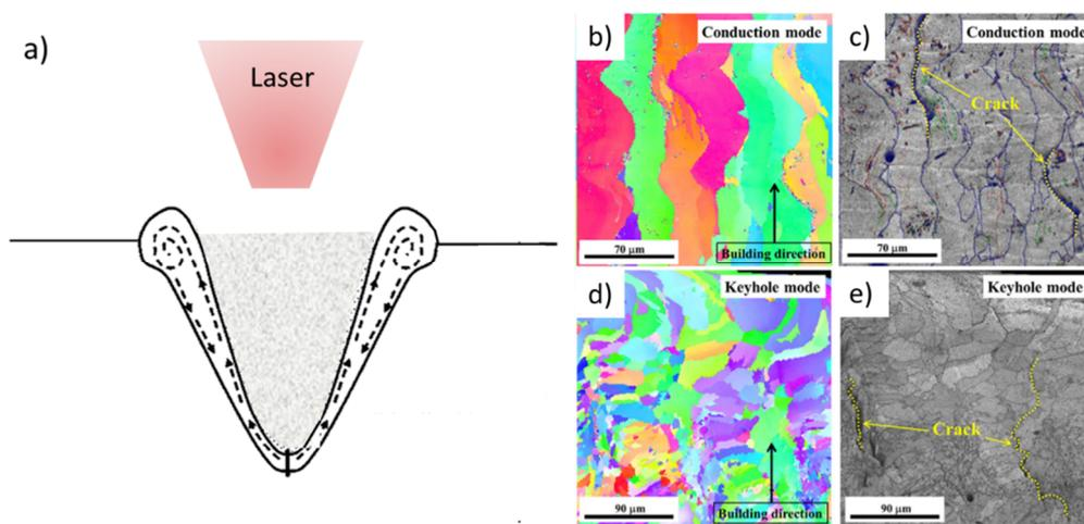
**Figure 6.** (a) Schematic representation of a keyhole melting and EBSD maps of 7050 samples produced in (b,c) a conduction melting mode and (d,e) a keyhole melting mode. (b,d) orientation image map and (c,e) grain boundary misorientation angle map. Adapted from [59], with permission from © 2017 Elsevier.
