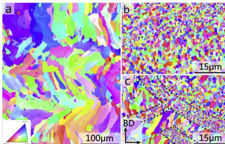
**Figure 7.** EBSD inverse pole figure (IPF) maps of Al-Cu-Mg fabricated at  $v = 5$  m/min (a) and Zr/Al-Cu-Mg sample fabricated at  $v = 5$  m/min (b) and  $v = 15$  m/min (c), respectively. Adapted from [34], with permission from © 2017 Elsevier.
