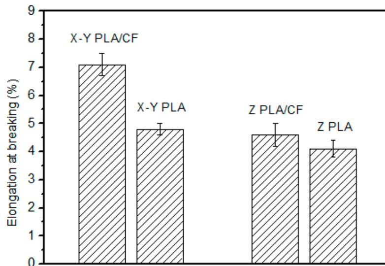
Figure 4. At breaking of the polylactic acid–carbon fiber (PLA–CF) specimens.
