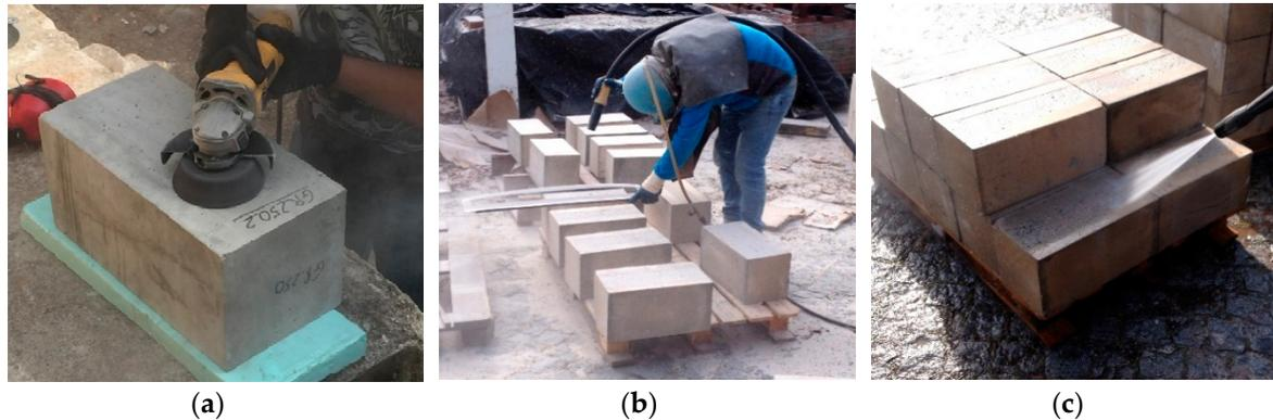
Figure 2. Concrete surface preparation: (a) grinding; (b) sandblasting; (c) surface cleaning.
