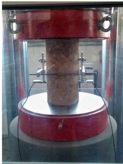
**Figure 9.** Testing setup of the static modulus of elasticity.
