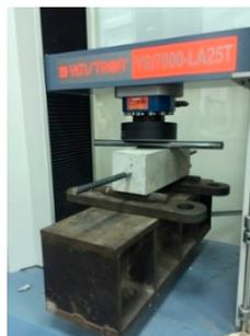
**Figure 16.** Pre-cracking of the beam specimen by the bending method.
