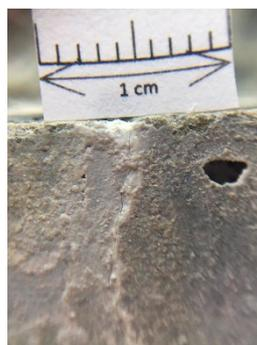
**Figure 21.** Surface crack of the concrete specimen.
