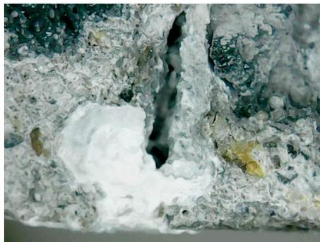
Figure 23. Thickness observation of the vertical section crack repair under a portable microscope (100 times magnification).
