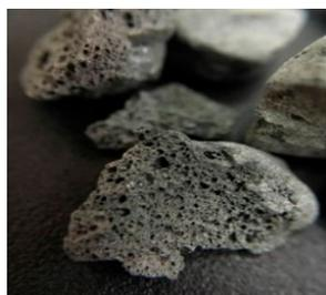
**Figure 1.** Appearance of lightweight expanded shale aggregates.
