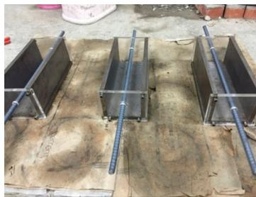
Figure 11. Mold of the beam specimen.
