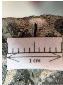
Figure 22. Crack repair of the concrete specimen.
