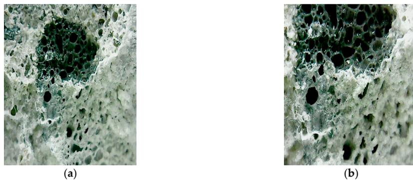
**Figure 20.** Sectional observation of experimental group II under a portable microscope: (a) 100 times magnification; (b) 200 times magnification.
