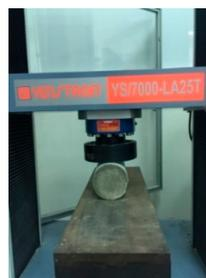
Figure 12. Pre-cracking of the concrete cylindrical specimen by the splitting method.
