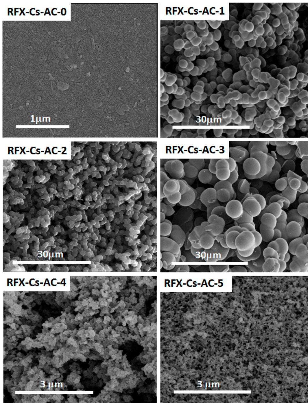
Figure 2. NanoSEM photomicrographs of RFX-Cs-AC samples.
