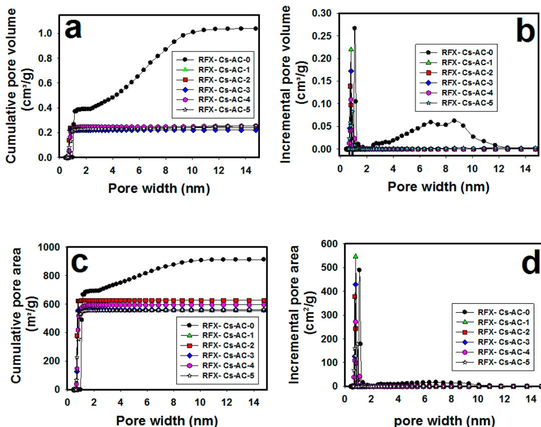
**Figure 4.** Relationships of (a) cumulative pore volume, (b) incremental pore volume, (c) cumulative pore area and (d) incremental pore area versus pore widths of different RFX-Cs-AC samples.
