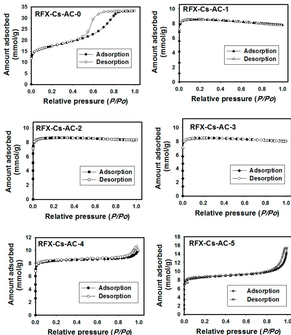
Figure 3. Adsorption/desorption isotherms of N<sub>2</sub> gas at 77 K onto RFX-Cs-AC samples.
