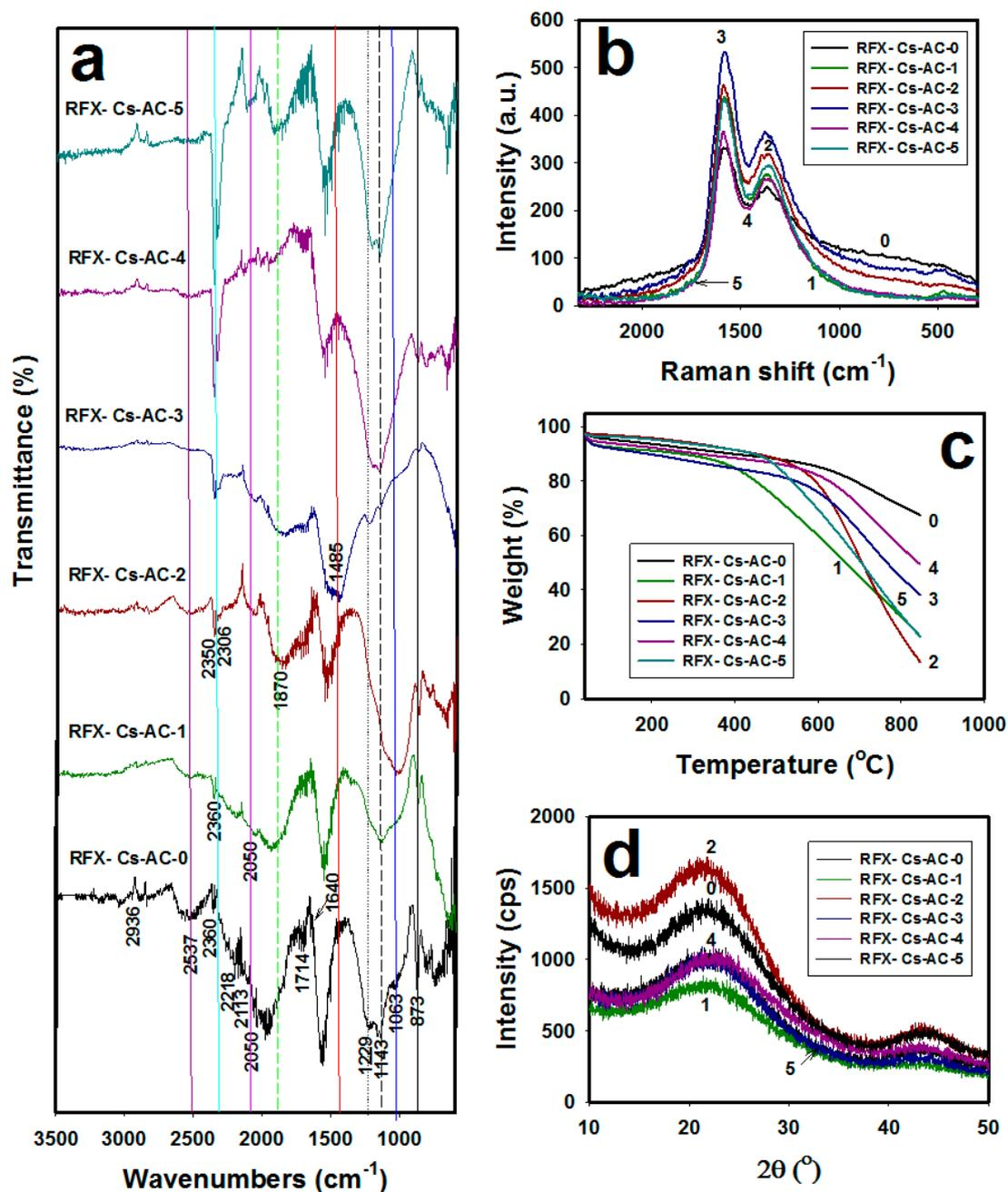
**Figure 1.** (a) FTIR spectra, (b) Raman spectra, (c) TGA thermograms and (d) XRD patterns of RFX-Cs-AC samples. Curve numbers from 0 to 5 correspond to the suffix numbers of RFX-Cs-AC samples.
