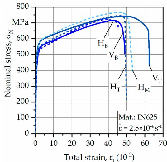
Figure 6. Averaged results of tensile tests.
