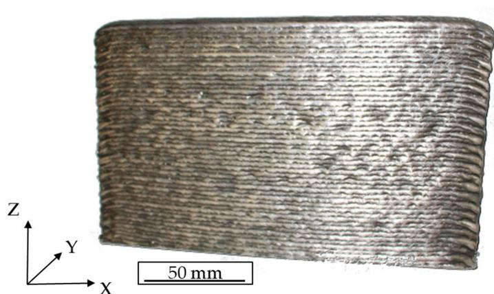
**Figure 1.** As-deposited arc-welded nickel-based superalloy Inconel 625 (IN625).
