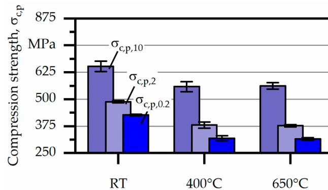
**Figure 8.** Compression strength  $\sigma_{c,p}$  for the investigated materials at different temperatures.
