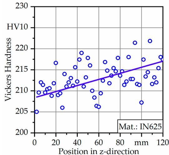
**Figure 5.** Hardness profile of IN625 along the building direction in a cross section (Y–Z plane).
