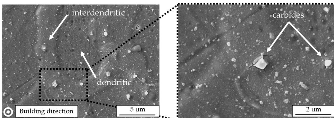
**Figure 4.** Scanning electron microscope images of arc-welded IN625 perpendicular to the building direction.
