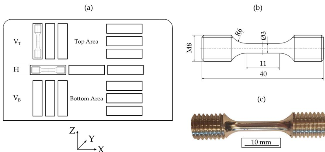
**Figure 2.** Schematic configuration of tensile specimens: (a) positions, (b) dimensions (in mm), and (c) final geometry.
