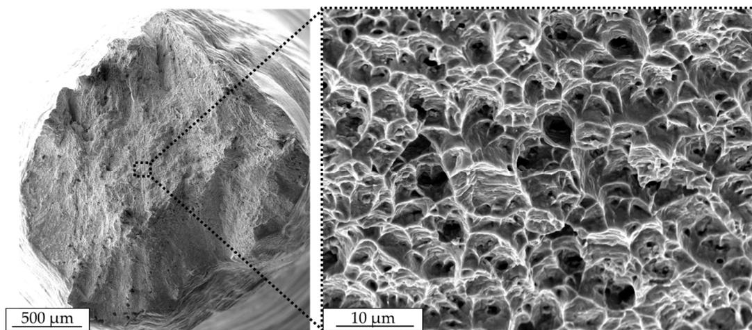
**Figure 9.** Fracture surface with the corresponding magnification of IN625 after a tensile test in the scanning electron microscope.
