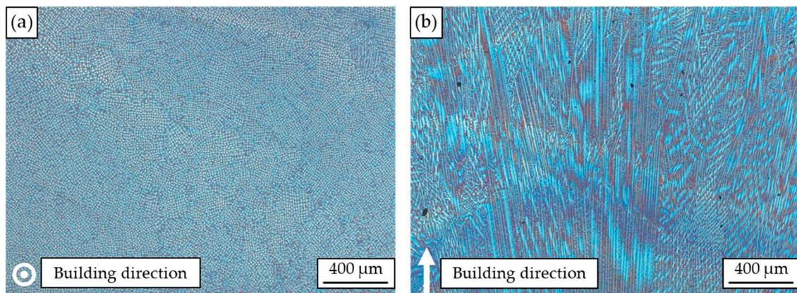
**Figure 3.** Optical microscope images of arc-welded IN625: cross section (a) perpendicular and (b) parallel to the building direction.
