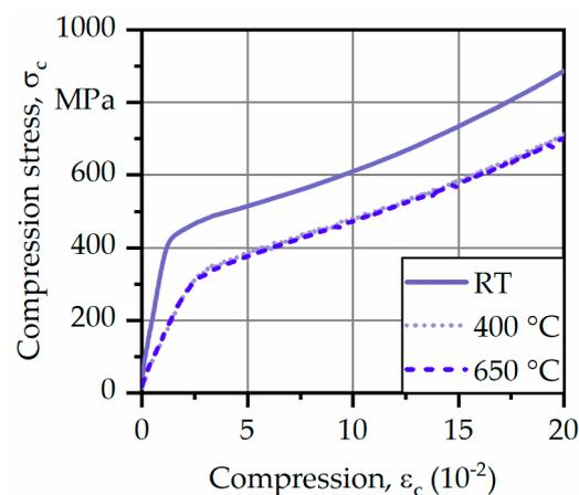
Figure 7. Averaged results of compression tests. RT: room temperature.
