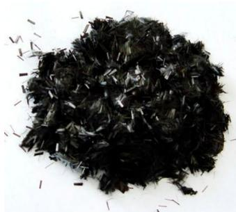
**Figure 3.** Short-cut carbon fibers.
