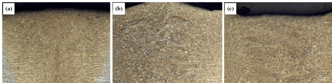
Figure 6. 200× metallographic photos of welds obtained at different laser power: (a) 1.1 kW, (b) 1.8 kW, and (c) 2.7 kW.
