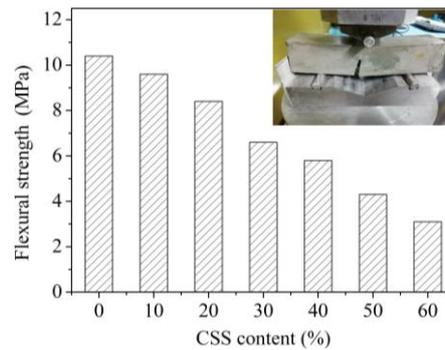
**Figure 8.** Flexural strength of the sample.
