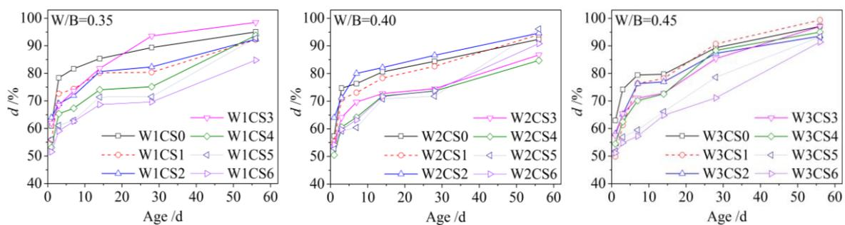
Figure 4. Hydration degree of the sample at a different age.
