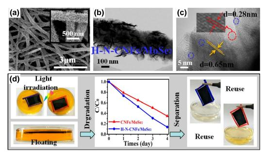
**Figure 6.** (a) SEM images, (b,c) Transmission electron microscopy (TEM) images of H–N–CNF/MoSe<sub>2</sub> heterojunctions. (d) Digital photographs demonstrating the self-supporting photocatalysis application of H–N–CNF/MoSe<sub>2</sub> and CNFs/MoSe<sub>2</sub>. Adapted with permission from Reference [124]. Copyright (2018) American Chemical Society.
