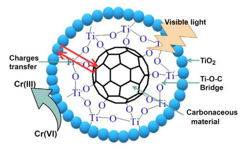
**Figure 2.** Schematic of proposed degradation of pollutants with TiO<sub>2</sub>/carbon composites. Adapted with permission from Reference [63]. Copyright (2019) Elsevier.
