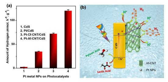
**Figure 5.** (a) Comparison of hydrogen production with Pt nanoparticle-loaded materials versus pure CdS. (b) Schematic illustration demonstrating mechanism of H<sub>2</sub> production via photocatalytic water splitting by Pt–Af–CNT/CdS ternary composite. Adapted with permission from Reference [109]. Copyright (2018) Elsevier.
