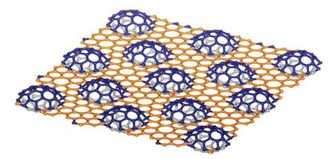
**Figure 9.** Schematic illustration showing the structures of various bubble-wrap allotropes. Adapted with permission from Reference [141]. Copyright (2018) Royal Society of Chemistry.
