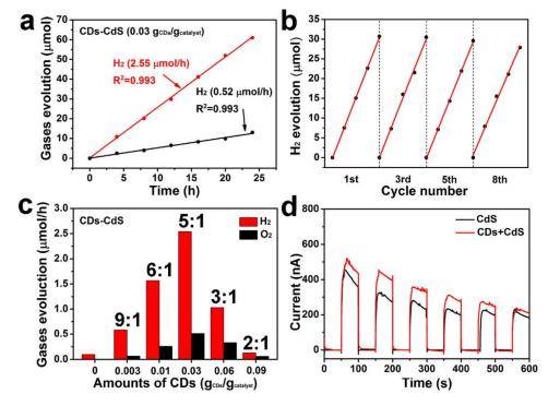
**Figure 4.** (a) Water splitting performance of the carbon dots (CDs)–CdS under visible light irradiation. (b) The cyclic stability of visible light photocatalytic water splitting performance of CDs–CdS. (c) The amount of produced gases of CDs–CdS with different content of CDs. (d) Photoresponse properties of pristine CdS and representative CDs–CdS. Adapted with permission from Reference [85]. Copyright (2017) Elsevier.
