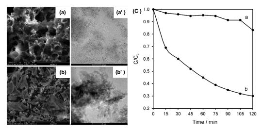
**Figure 7.** (**a**,**b**) SEM, (**a'**,**b'**) TEM of pristine GQDs and NiAl<sub>2</sub>O<sub>4</sub>/GQDs composite, respectively. (**c**) Photodegradation performances of NiAl<sub>2</sub>O<sub>4</sub> (line a) and NiAl<sub>2</sub>O<sub>4</sub>/GQDs composite (line b) over the Rhodamine B (RhB). Adapted with permission from Reference [136]. Copyright (2019) MDPI AG.
