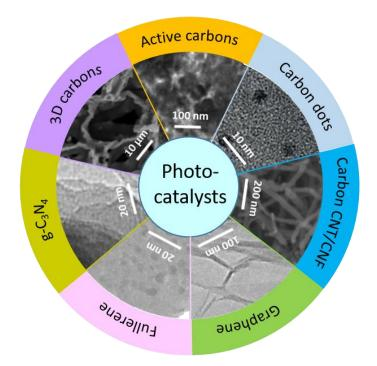
Scheme 1. Carbonaceous materials for photocatalysts. Adapted with permission from Reference [35] Copyright (2017) Springer; [36] Copyright (2018) Wiley; [37] Copyright (2018) Springer; [38] Copyright (2018) Wiley; [39] Copyright (2019) American Chemical Society; [40] Copyright (2018) Elsevier; [41] Copyright (2019) Elsevier.
