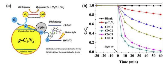
**Figure 10.** (a) Schematic illustration showing the visible light-induced photocatalytic degradation of organic compounds over CQD-modified g-C<sub>3</sub>N<sub>4</sub>. (b) Photocatalytic degradation kinetics of diclofenac by different photocatalysts. Adapted with permission from Reference [155]. Copyright (2019) Elsevier.
