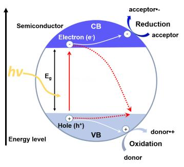
**Figure 1.** Schematic illustration demonstrating the photocatalytic process of a semiconductor photocatalysts. Adapted with permission from Reference [22]. Copyright (2011) Elsevier.
