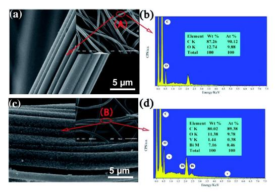
**Figure 3.** SEM images (**a**,**b**) and corresponding EDS spectra (**c**,**d**) original activated carbon fibers (ACFs) and BiVO<sub>4</sub>@ACFs. Adapted with permission from Reference [79]. Copyright (2018) Royal Society of Chemistry.
