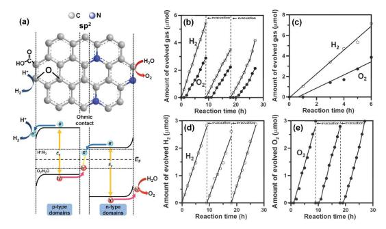
**Figure 8.** (a) Schematic illustration of the configuration and energy diagram for a NGO–QD photochemical diode. Visible light induced photocatalytic water splitting performance over different photocatalysts: (b) 1.2 g of NGO–QDs, (c) 0.5 g of Rh<sub>2–y</sub> Cr<sub>y</sub>O<sub>3</sub>/GaN:ZnO, (d) 1.2 g of GO–QDs, (e) 1.2 g of NH<sub>3</sub>–NGO–QDs. Adapted with permission from Reference [138]. Copyright (2014) Wiley.
