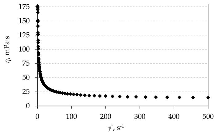
**Figure 4.** Plot of apparent viscosity ( $\eta$ ) versus increasing shearing rate ( $\dot{\gamma}$ ) for 70 wt.%  $\text{Al}_2\text{O}_3$  water based suspension which contains 20 dwb.% of waste  $\text{Al}_2\text{O}_3$  powder, with optimal amounts of additives.
