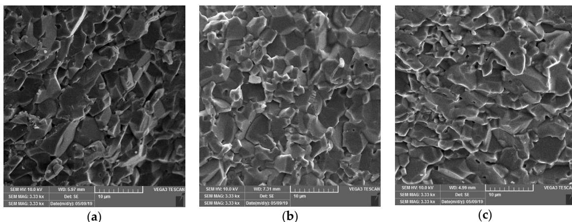
**Figure 3.** SEM images of alumina morphology sintered at 1550 °C with fixed weight ratios of waste alumina powder of 20 wt.%, 0.05 wt.% Tiron and 0.1 wt.% PVA and with varying amounts of magnesium aluminate spinel: (a) 0.2 wt.% MgAl<sub>2</sub>O<sub>4</sub>, (b) 0.6 wt.% MgAl<sub>2</sub>O<sub>4</sub> and (c) 1.0 wt.% MgAl<sub>2</sub>O<sub>4</sub> expressed on dry weight basis.
