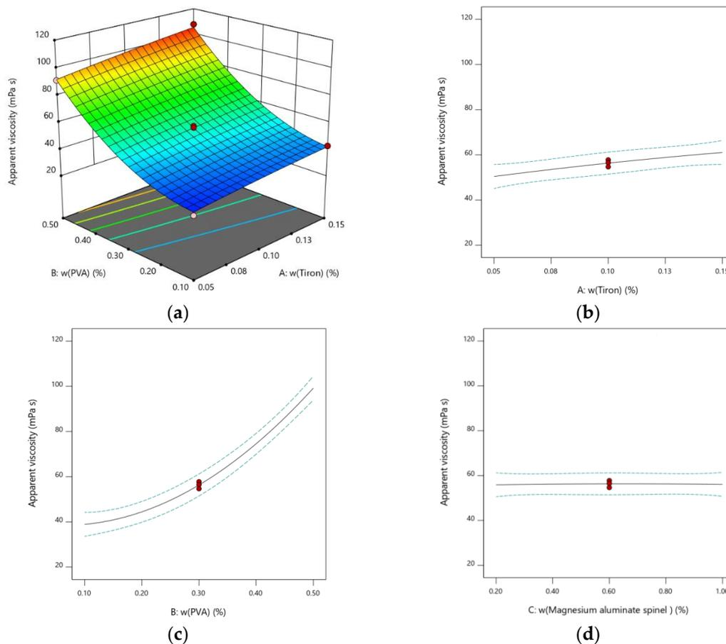
**Figure 2.** The effect on apparent viscosity of 70 wt.%  $\text{Al}_2\text{O}_3$  suspensions which contain 20 dwb.% waste  $\text{Al}_2\text{O}_3$  powder: (a) 3D-plot of viscosity on two factors (PVA content and Tiron content); (b) Tiron; (c) poly (vinyl alcohol) (PVA); (d) magnesium aluminate spinel ( $\text{MgAl}_2\text{O}_4$ ).
