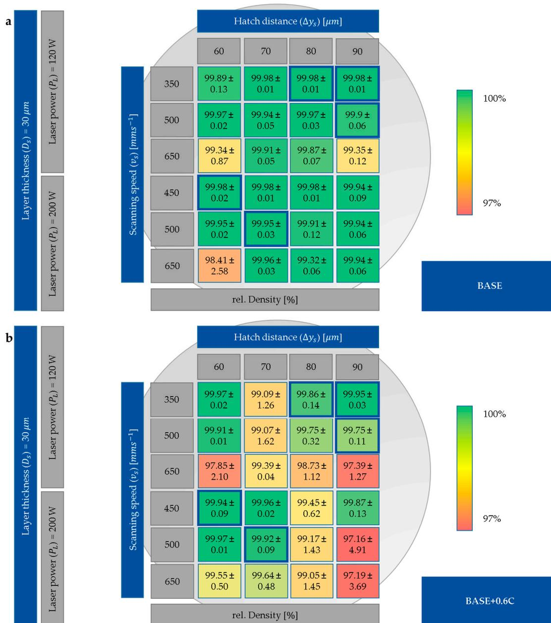
**Figure 4.** Color-coded relative densities dependent on different process parameters for (a) BASE and (b) BASE + 0.6C. The selected parameter sets for further production of samples are marked in blue.
