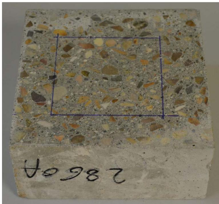
**Figure 2.** Surface of analysis drawn on the polished surfaces of a cubic sample.
