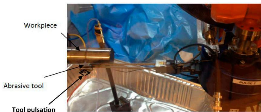
Figure 1. Robot-Assisted Polishing (RAP) machine.
