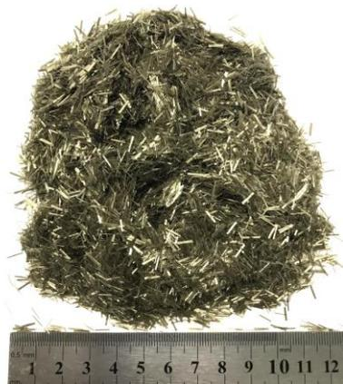
**Figure 1.** Morphology of basalt fiber with length of 6 mm in this study.
