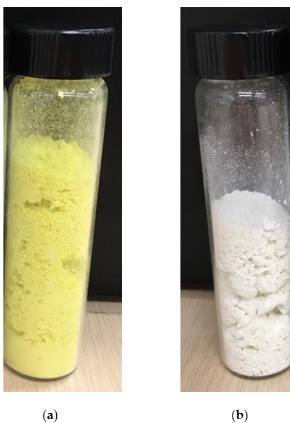
Figure S1. Images of (a) caesium phosphomolybdate (CPM) formed at 50 °C displaying a yellow coloured solid and (b) zirconium molybdate (ZM-a) displaying a white coloured solid.
