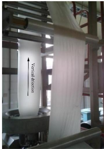
Figure 3. Continuous and stable blowing of HPDSP-OMMT film.
