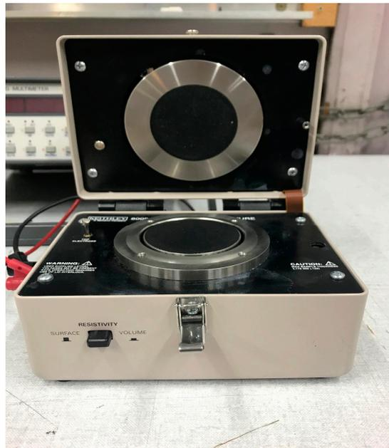
**Figure 1.** Photo of KEITHLEY 8009 resistivity test fixture.
