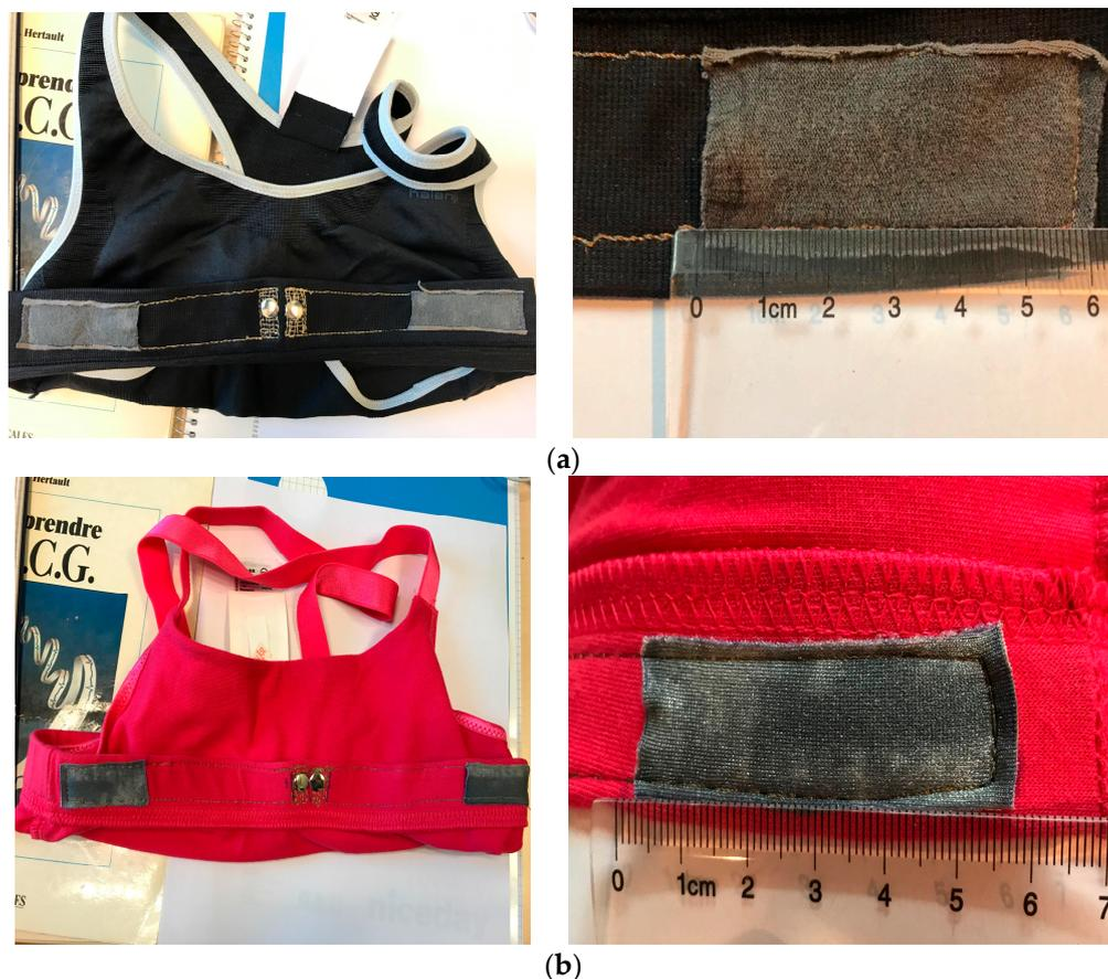
**Figure 4.** (a) Cotton electrodes sewn into bras; (b) Polyamide electrodes sewn into bras.
