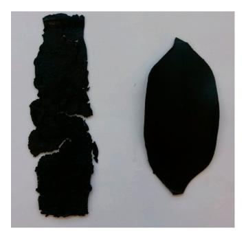
Figure 20. Materials MU2 (left) and MU3 (right) after pressing at same conditions.
