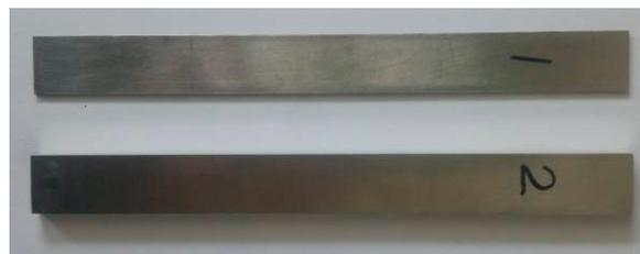
**Figure 9.** Waveguide bars named No. 1 and No. 2 (the thickness of No. 1 is 1 mm, and the thickness of No. 2 is 4 mm).
