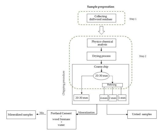
Figure 3. Schematic procedure.
