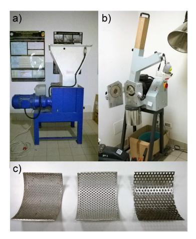
$Figure\ 2.\ (a)\ \text{Loose chips wood shredder;}\ (b)\ \text{Refining mill;}\ (c)\ \text{Refining mill grids}.$
