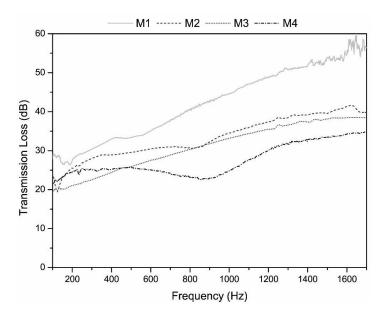
**Figure 15.** Transmission loss of the mineralized samples.
