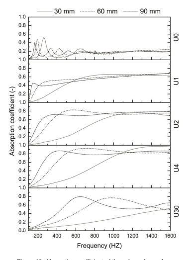
Figure 12. Absorption coefficient of the unbound samples.
