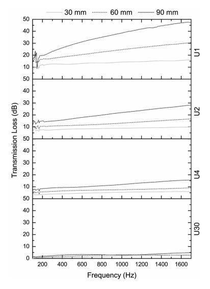
Figure 14. Transmission loss of the unbound samples.
