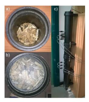
**Figure 10.** (a,b) Specifically designed sample holder; and (c) Tube configuration for transmission loss measurements.
