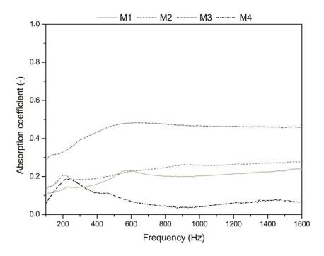
Figure 13. Absorption coefficient of the mineralized samples.
