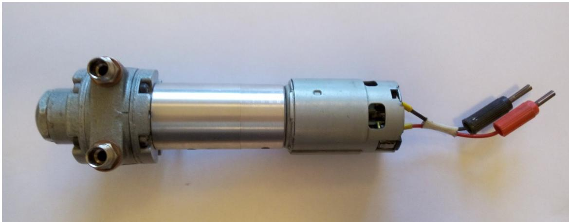
**Figure 9.** The view of the expander-generator unit disassembled from the test-stand.
