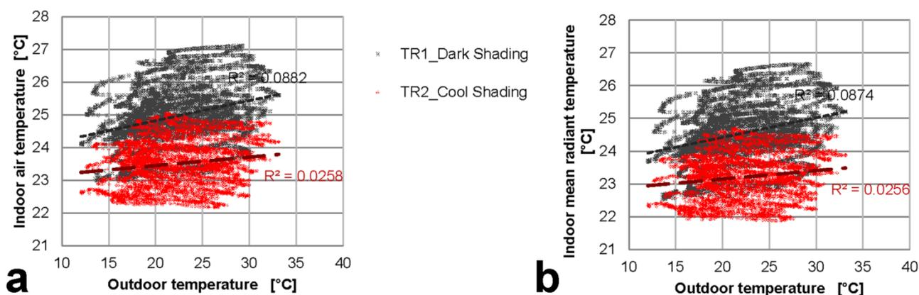
**Figure 9.** Indoor thermal comparative assessment of the two configurations in terms of (a) air temperature and (b) mean radiant temperature, in free floating conditions.
