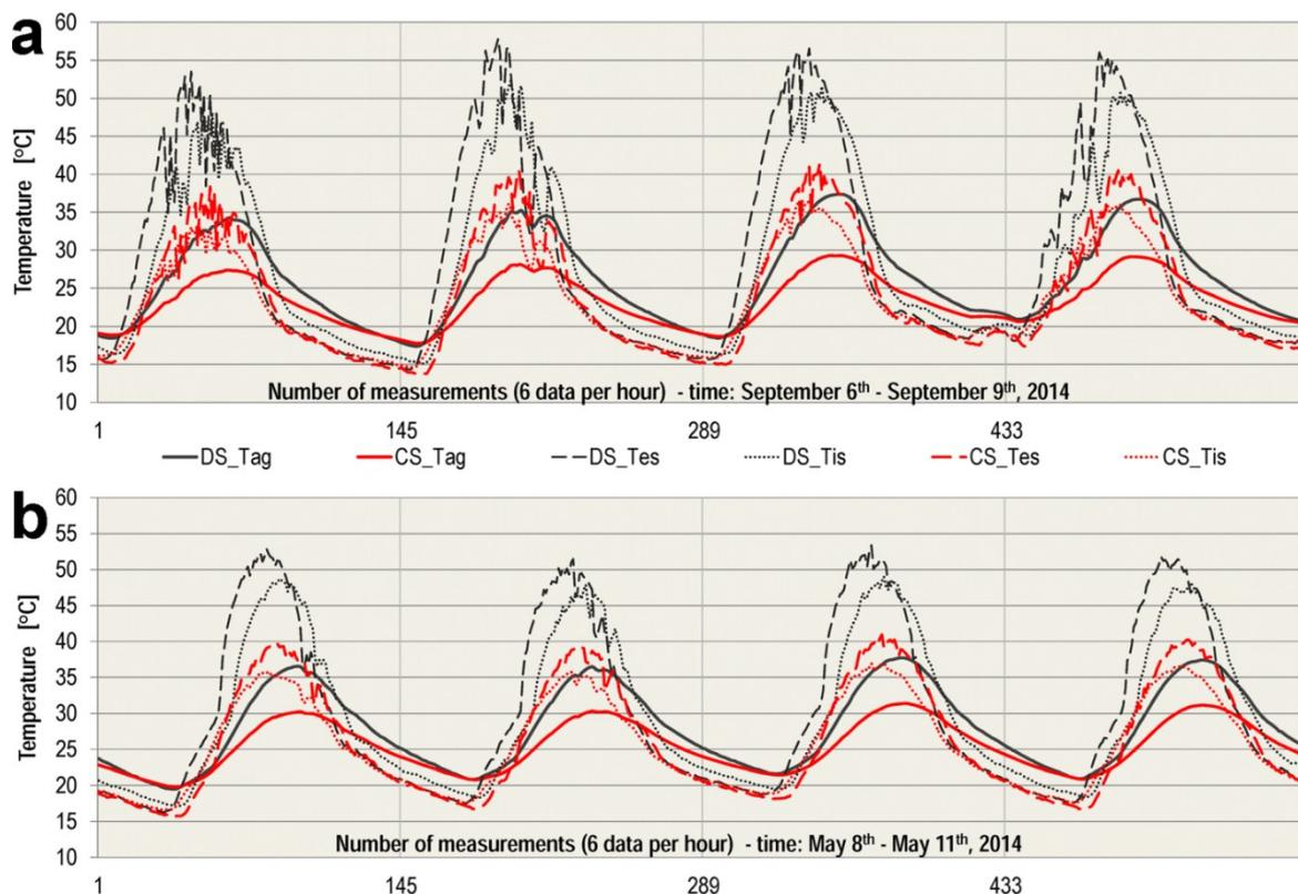
**Figure 6.** Indoor thermal behavior of the test-rooms before the implementation of the Cool Shading systems in TR2. (a) Summer conditions; (b) Spring conditions.
