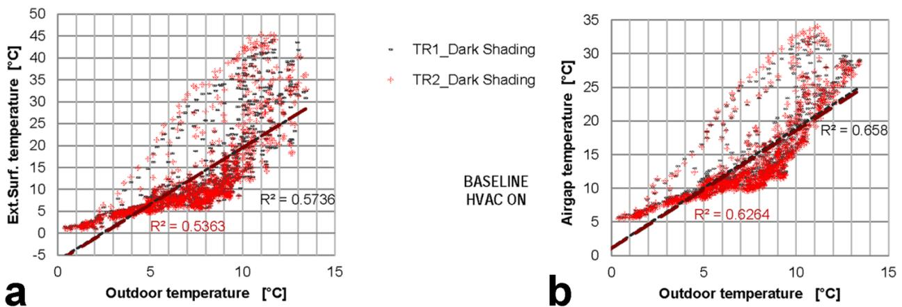
Figure 4. Shutter external surface temperature (a) and airgap temperature (b) of the two test-rooms vs. outdoor thermal conditions in baseline configuration.
