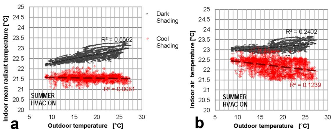
**Figure 8.** Indoor thermal comparative assessment of the two configurations in terms of (a) mean radiant temperature and (b) air temperature, when the HVAC system is operative.
