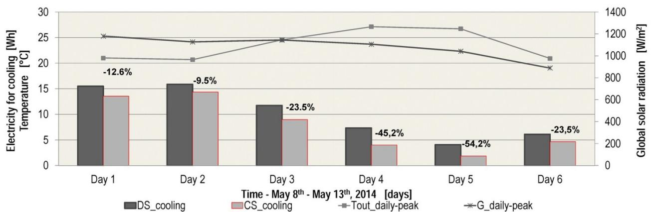
**Figure 10.** Daily energy requirement for cooling of CS and DS with varying daily weather parameters, *i.e.*, outdoor dry bulb temperature and global solar radiation.
