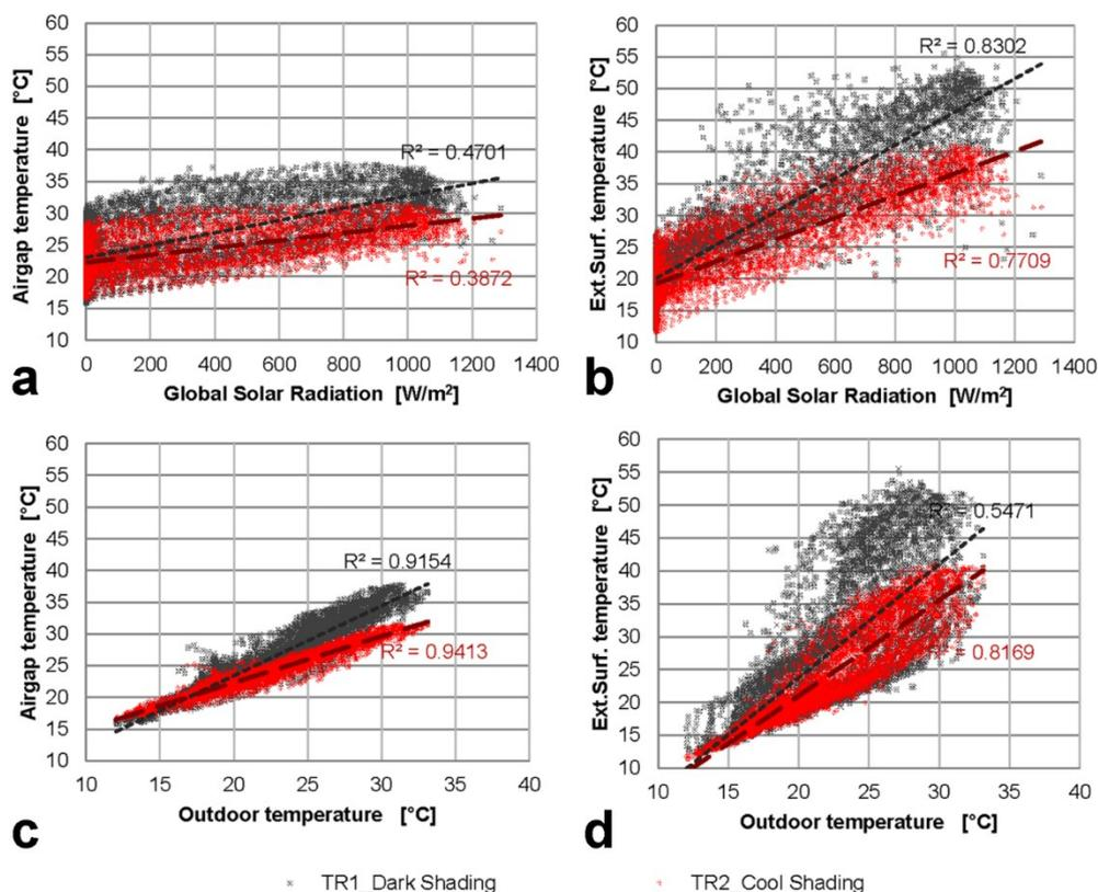
**Figure 7.** Air gap and surface temperature of the shutters vs. outdoor weather parameters. (a,b) Global solar radiation over an horizontal plane; (c,d) Outdoor dry bulb temperature.
