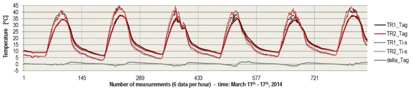
Figure 3. Thermal profiles of the monitored test-rooms during the baseline characterization.
