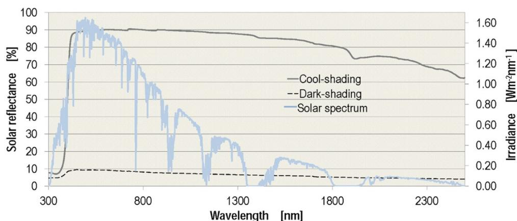
**Figure 2.** Spectrophotometer measurement results of solar reflectance of Cool Shading vs. Dark Shading.
