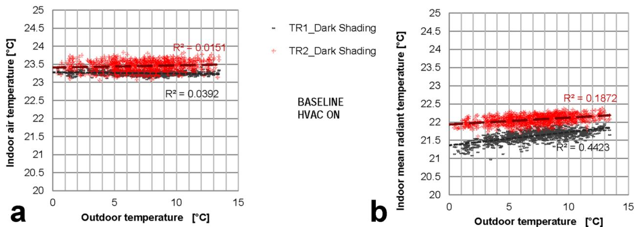
**Figure 5.** Indoor thermal behavior of the test-rooms before the implementation of the Cool Shading systems in TR2. Indoor air temperature trends (a), and mean radiant temperature trends (b).
