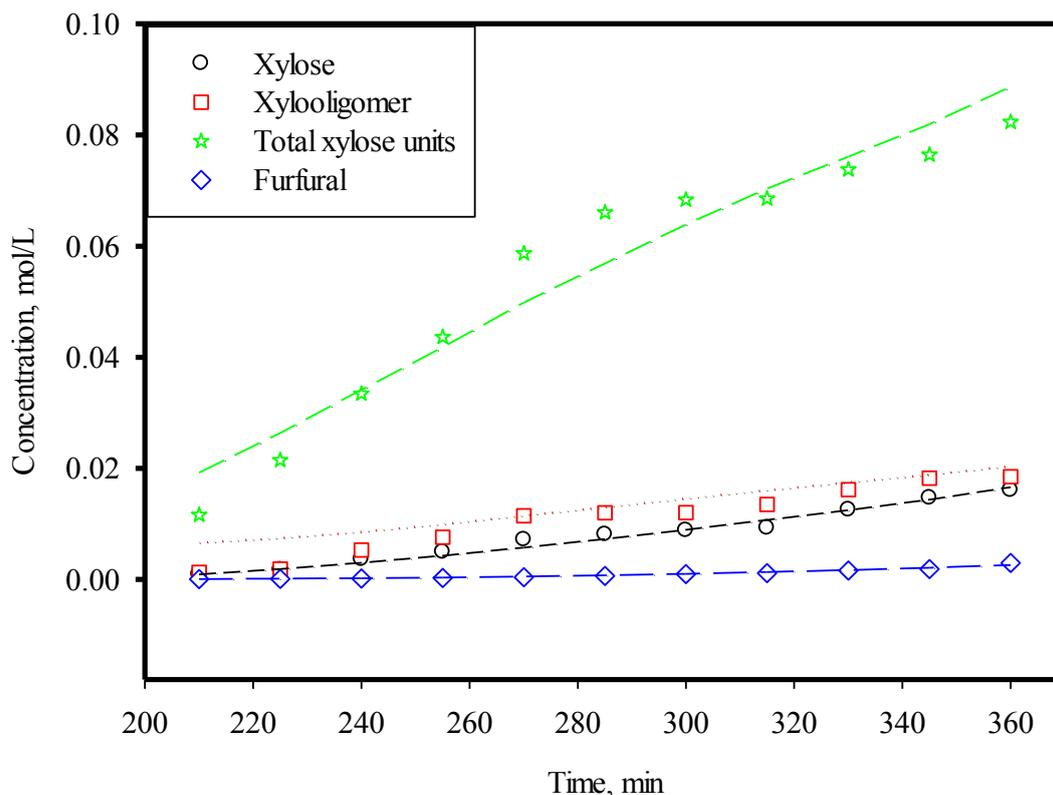
**Figure 5.** Variations of xylose, xylooligomer, total xylose units, and furfural as a function of extraction time. The lines are based on Equations (19)–(29).
