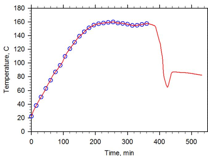
**Figure 1.** Temperature profile during the hot-water extraction of Northern Boreal Aspen woodchips, with symbols indicating the time at which extraction liquor samples are taken.
