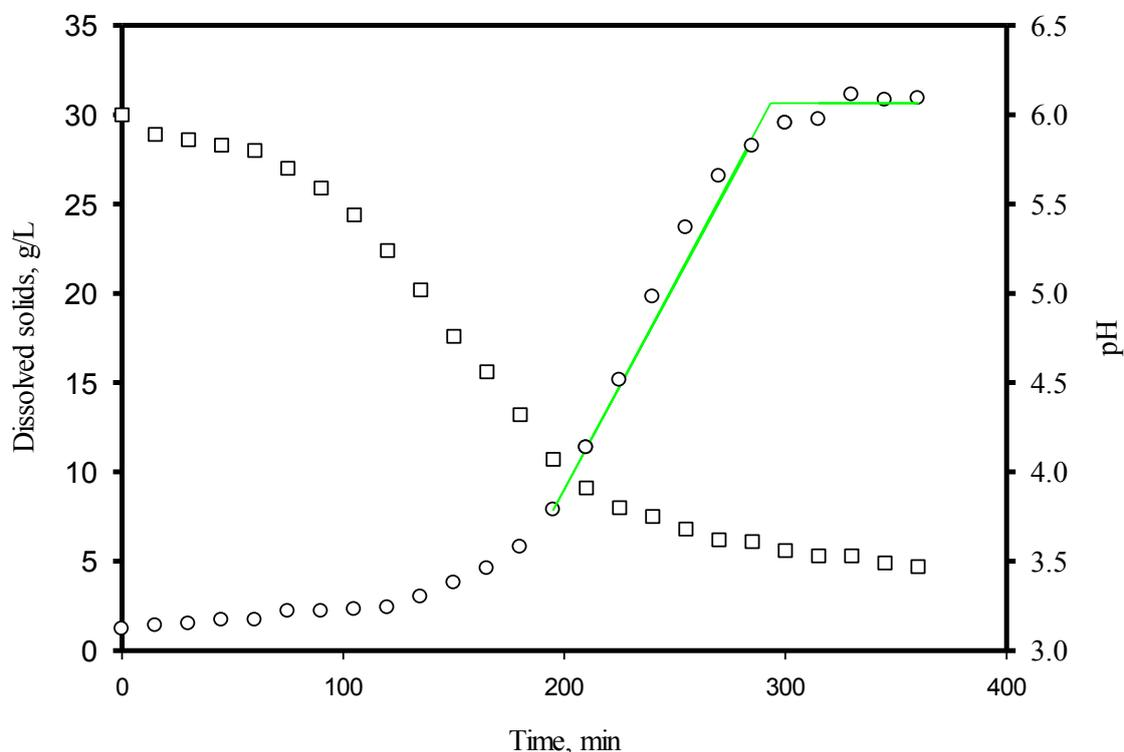
**Figure 3.** Variations of dissolved solids and pH during hot water extraction of aspen. Square ( $\square$ ) represent pH. Circle ( $\circ$ ) represents dissolved solid. The lines are based on Equation (4). The  $K_{ED}$  is  $288.4 \text{ g}\cdot\text{min}^{-1}$ .
