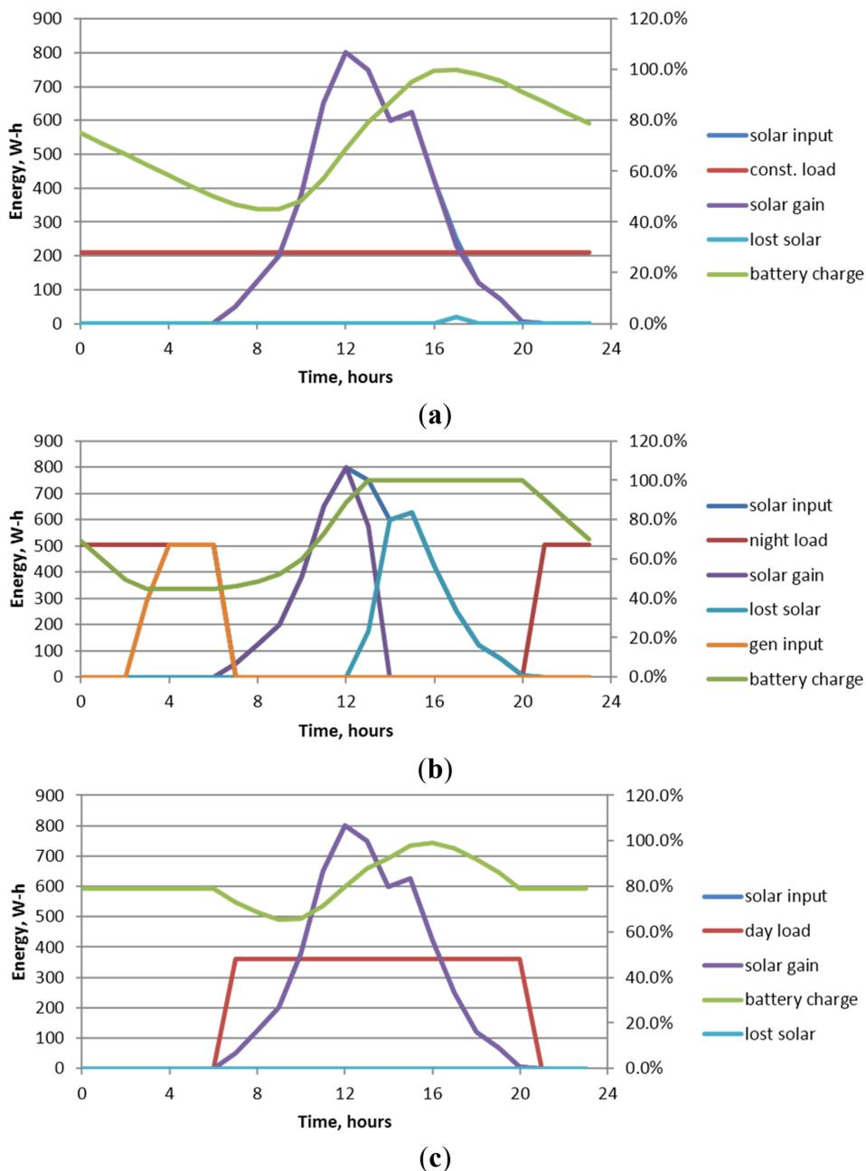
**Figure 3.** (a) Energy flows and state of battery bank charge for sunny day with constant electrical load over 24 hours; (b) Energy flows and state of battery bank charge for sunny day with constant electrical load concentrated during nighttime hours; (c) Energy flows and state of battery bank charge for sunny day with constant electrical load concentrated during daylight hours.
