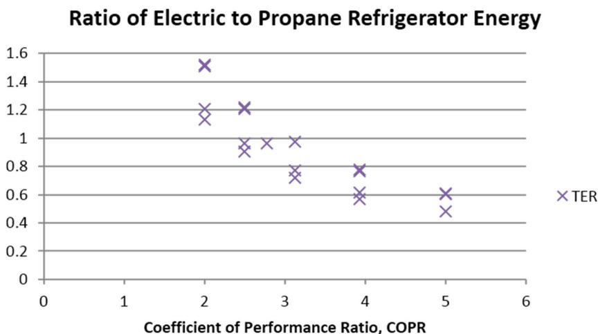
**Figure 6.** Ratio of electric refrigerator energy usage to propane refrigerator energy usage as a function of the Coefficient of Performance Ratio, COPR.
