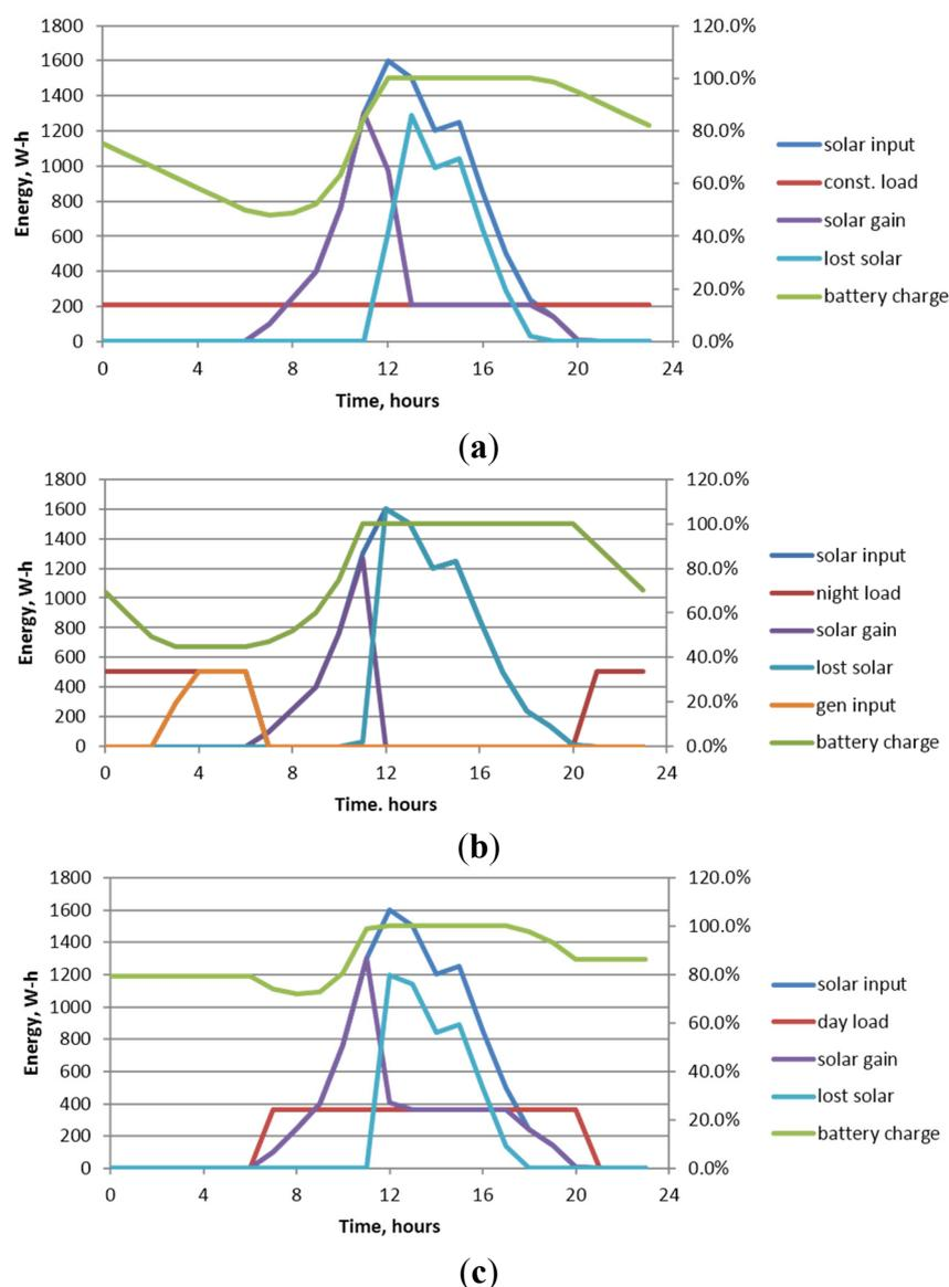
**Figure 4.** (a) Energy flows and state of battery bank charge for sunny day with constant electrical load over 24 hours with double the solar input; (b) Energy flows and state of battery bank charge for sunny day with constant electrical load concentrated during nighttime hours with double the solar input; (c) Energy flows and state of battery bank charge for sunny day with constant electrical load concentrated during daylight hours with double the solar input.
