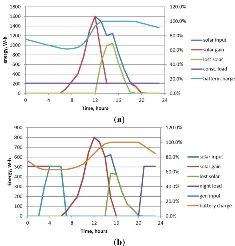
**Figure 5.** (a) Energy flows and state of battery bank charge for sunny day with constant electrical load over 24 h with double the solar input and double the battery bank storage capacity; (b) Energy flows and state of battery bank charge for sunny day with constant electrical load concentrated during nighttime hours with double the battery bank storage capacity.
