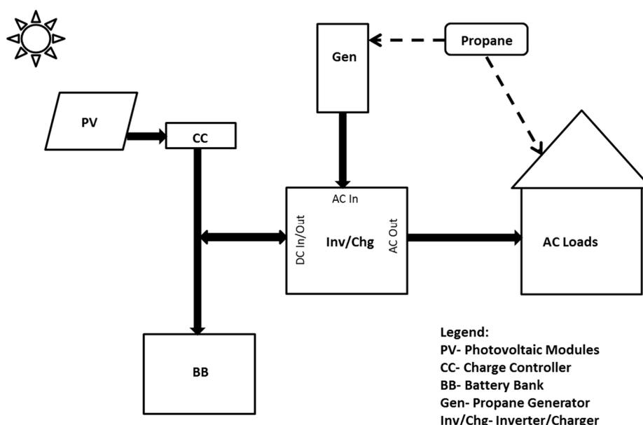
**Figure 1.** Typical off-grid, hybrid residential electrical power system.
