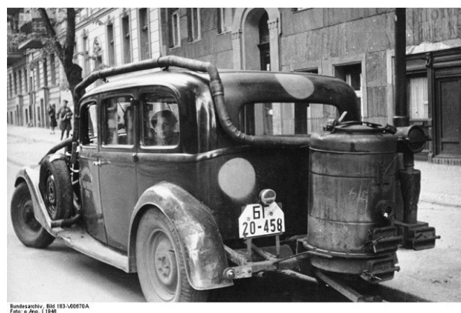
Figure 1. A WWII car with woodgas generator [4].
