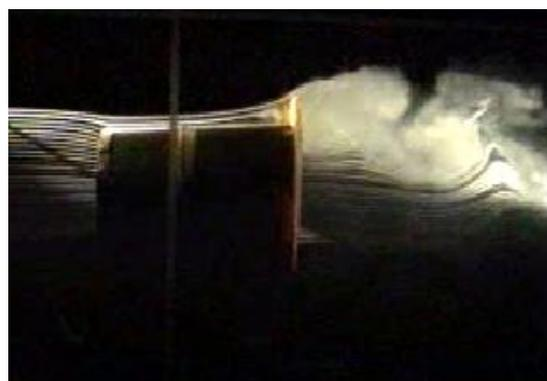
**Figure 5.** Flow around a wind turbine with brimmed diffuser (wind-lens).
