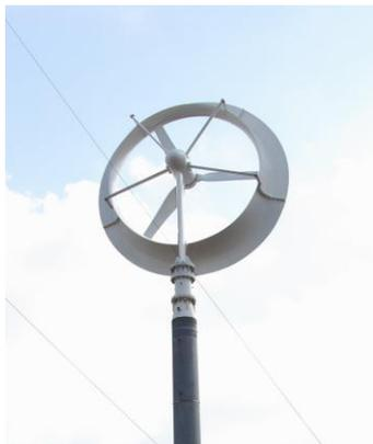
**Figure 15.** Field experiment of 5 kW wind-lens turbine.  $C_w$  is the power coefficient.  $C_w^* = 0.54$ , based on the brim diameter area.
