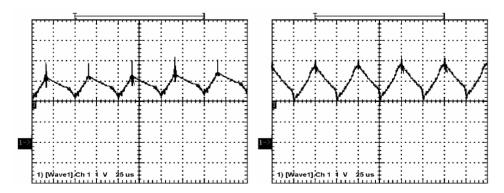
From Figure 14, it can be concluded that the charging current to both the main and auxiliary source was stable, with quick response and minor stability issues. In the emergent brake mode, the charging current to the main source can't hold the maximum value and begins to descend with overshoot.
