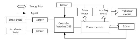
Figure 1. The schematic of the energy recovery system for the main and auxiliary sources.
