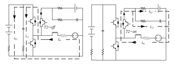
When the voltage of the EMF is not high enough to boost to the voltage of the main source, IGBT T2 switches on. The inductance begins to deliver the energy to the auxiliary source by the power converter working as a bucker. The current is along the positive polarity of EMF $\rightarrow$ T2 $\rightarrow$  the auxiliary source $\rightarrow$ the negative polarity of EMF, which is shown in Figure 5b. The value of the charging current to the auxiliary source depends on the duty cycle of PWM T2.
