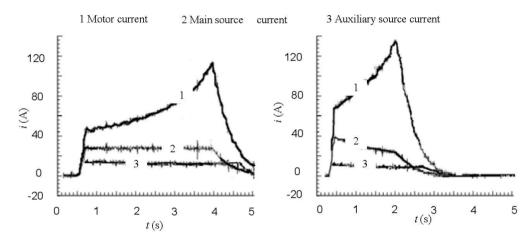
The experimental results show that the electrical circuit of the energy recovery system can work as a boost-buck converter. It can make the inductance of the motor pump the current to the main source and charge the auxiliary source at the same time. The simulated and experimental results showed that the current can be controlled, which validates the effectiveness and the feasibility of the proposed energy recovery system.
