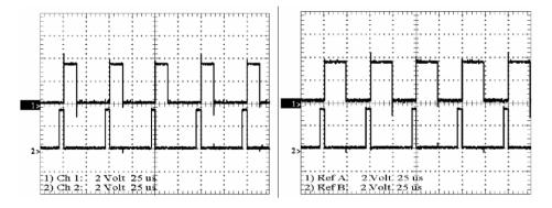
With the constraint of only two channels of Tektronix oscilloscope TEK2010, the motor currents corresponding to Figure 12 are shown in Figure 13. The motor current began to increase when T1 was switched on, then decreased when T1 was switched off. When T2 switched on, the rate of decrease was accelerated. The experimental results were in agreement with the simulated results in Figure 7.
