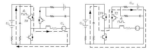
During the braking, the rotating motor can't stop suddenly because of its mechanical inertia and tends to rotate in the original direction. The EMF of the motor armature continues to hold its magnitude and polarity, the motor works in an energy resuming braking mode and a regenerative braking mode alternatively.
