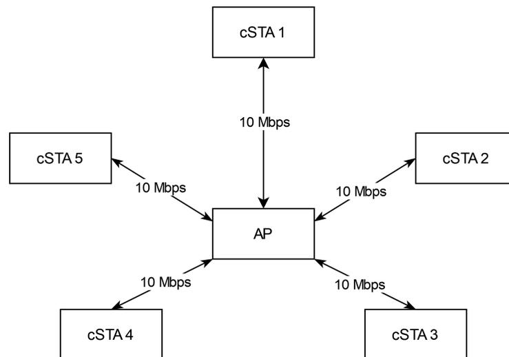
**Figure 3.** Topology of the first simulation scenario.
