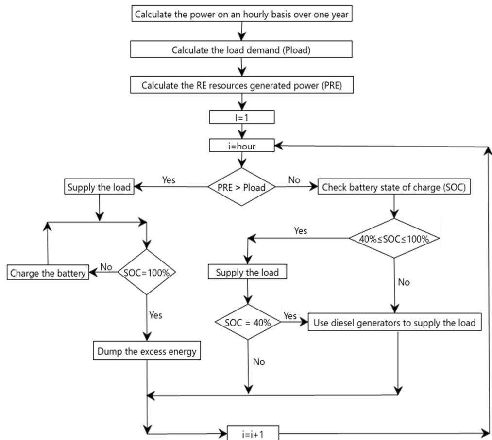
**Figure 6.** Flowchart depicting the operation of the system under various circumstances.
