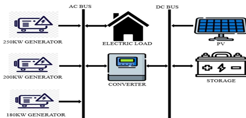
**Figure 5.** Proposed off-grid, RE-based hybrid system implemented in HOMER.
