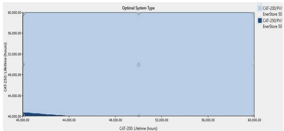
Figure 12. The effect of diesel generator lifespan on the optimized configuration.
