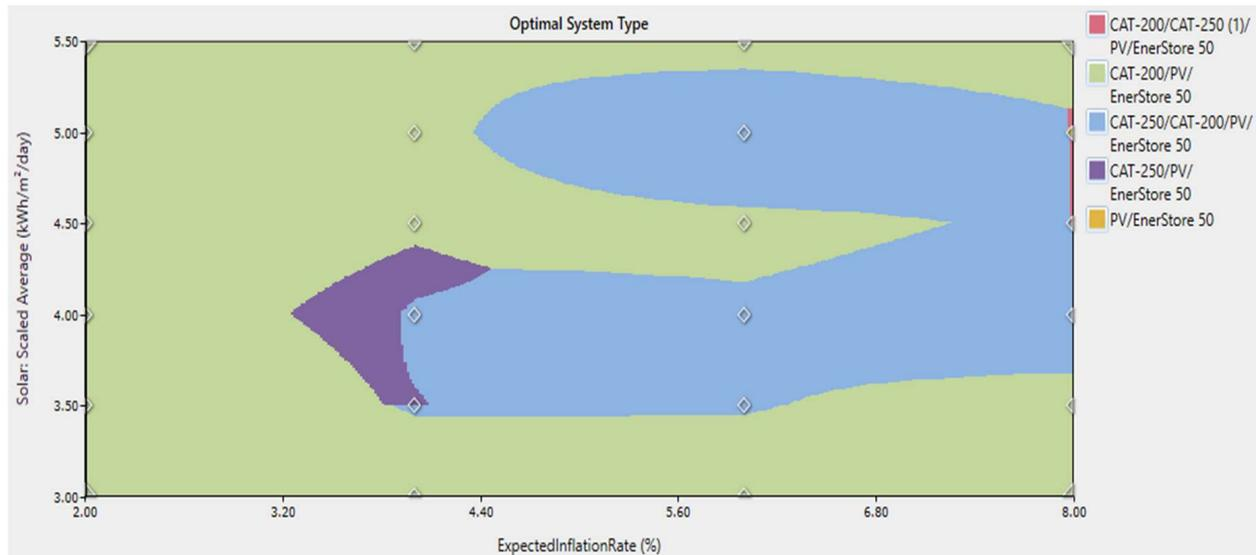
**Figure 9.** The influence of the inflation rate on the optimal system.
