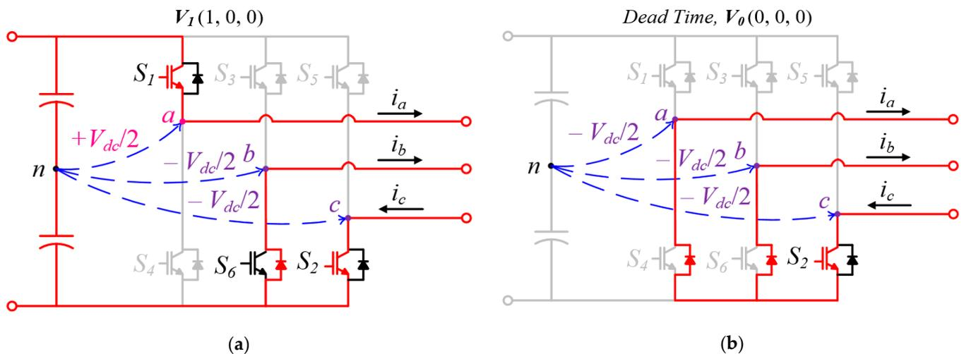
Figure 5. VV transition where the switch state becomes  $V_0$  during the dead time: (a) circuit configuration for  $V_1$  and (b) circuit configuration for dead time interval between  $V_1$  and  $V_3$ .
