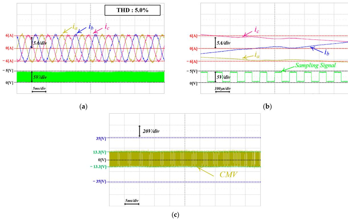
**Figure 18.** Experimental waveforms of FCS-MPC for CMV reduction using only non-ZVVs, considering dead time intervals (sampling frequency: 20 kHz): (a)  $i_a$ ,  $i_b$ ,  $i_c$ , and sampling signal; (b) magnified waveforms of (a); and (c) CMV.
