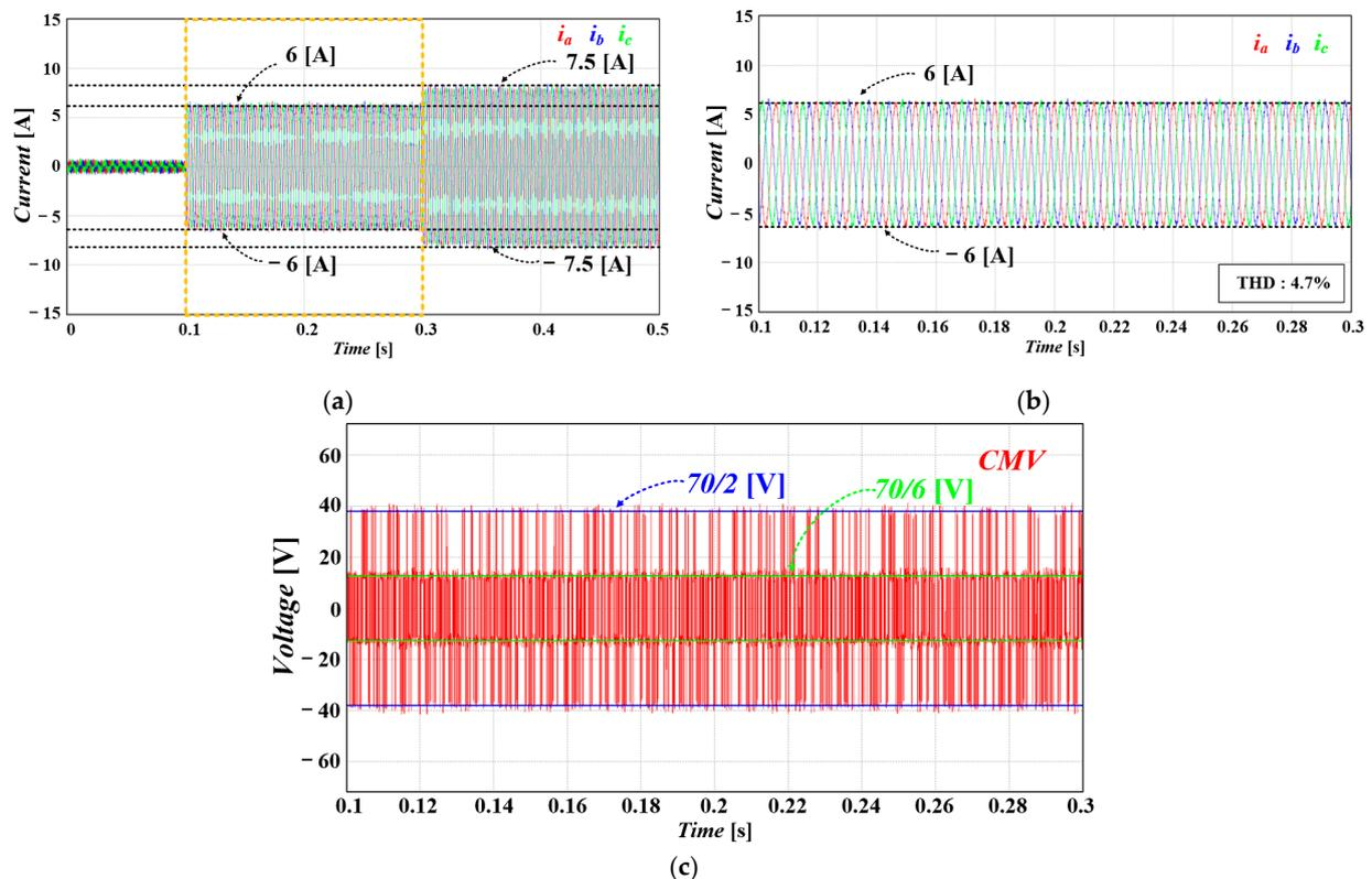
**Figure 10.** Simulation results of FCS-MPC for current control with both ZVVs and non-ZVVs applied: (a)  $i_a$ ,  $i_b$ , and  $i_c$ ; (b) magnified waveforms of (a); and (c) CMV.
