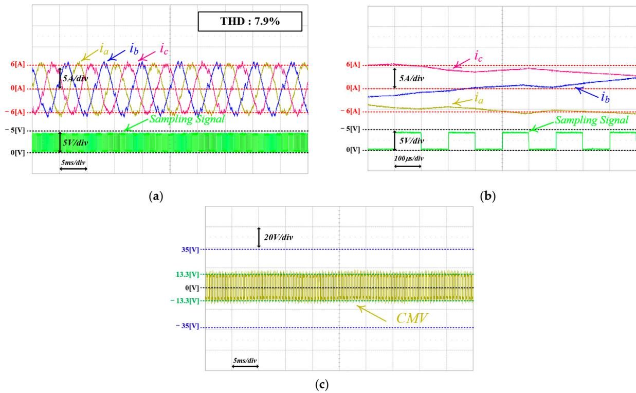
**Figure 17.** Experimental waveforms of FCS-MPC for CMV reduction using only non-ZVVs, considering dead time intervals (sampling frequency: 10 kHz): (a)  $i_a$ ,  $i_b$ ,  $i_c$ , and sampling signal; (b) magnified waveforms of (a); and (c) CMV.
