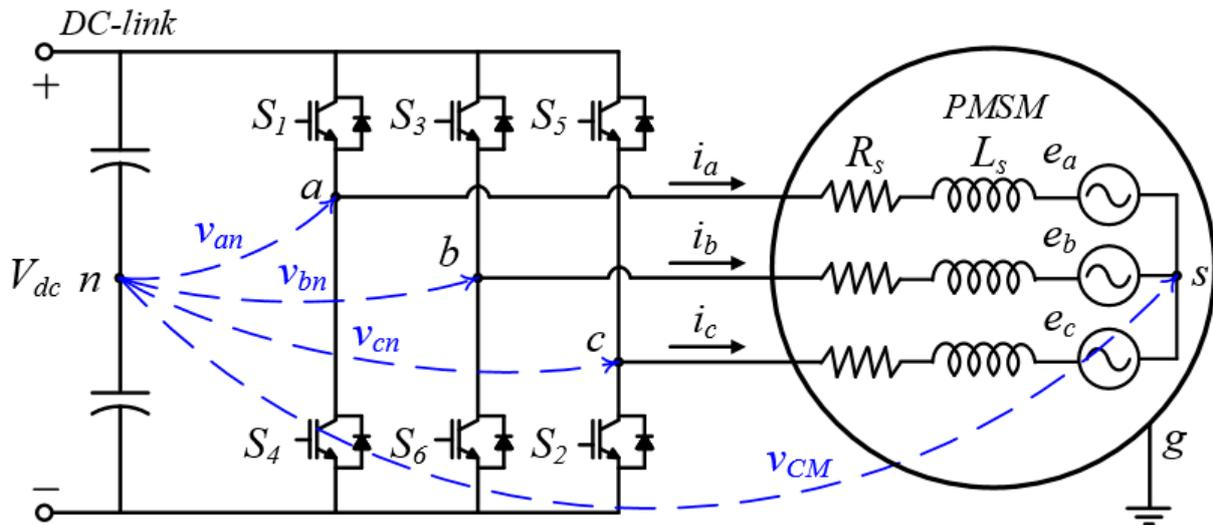
Figure 1. CMV in 2-level voltage source inverter.
