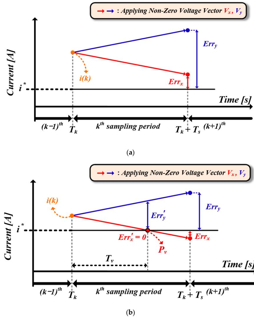
**Figure 7.** Cases where intersections between the predicted future current and the reference current are present and absent: (a) intersection absent and (b) intersection present.
