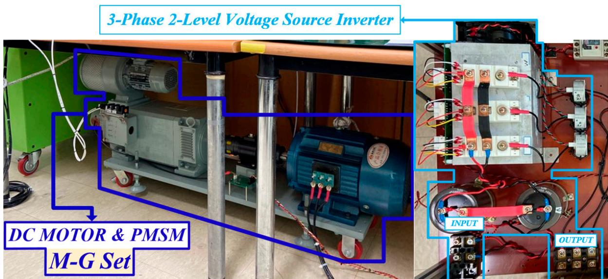
Figure 14. Experiment equipment and 2L-VSI.
