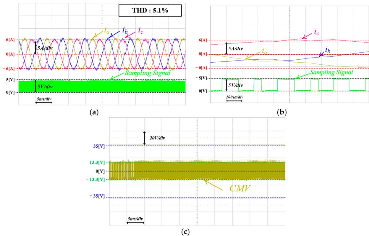
**Figure 19.** Experimental waveforms of the FCS-MPC with the proposed variable sampling frequency for CMV reduction: (a)  $i_a$ ,  $i_b$ ,  $i_c$ , and sampling signal; (b) magnified waveforms of (a); and (c) CMV.
