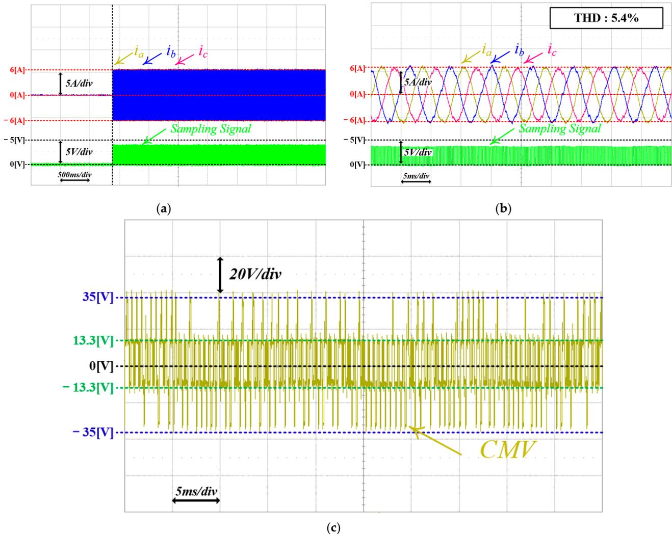
**Figure 15.** Experimental waveforms for FCS-MPC for current control: (a)  $i_a$ ,  $i_b$ ,  $i_c$ , and sampling signal; (b) magnified waveforms of (a); and (c) CMV.
