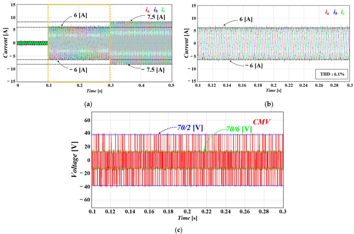
**Figure 11.** Simulation results of FCS-MPC using only non-ZVVs: (a)  $i_a$ ,  $i_b$ , and  $i_c$ ; (b) magnified waveforms of (a); and (c) CMV.
