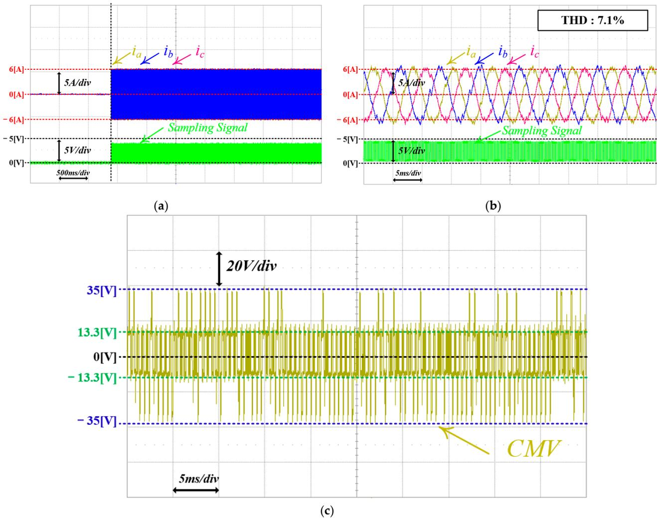
**Figure 16.** Experimental waveforms of FCS-MPC excluding ZVV: (a)  $i_a$ ,  $i_b$ ,  $i_c$ , and sampling signal; (b) magnified waveforms of (a); and (c) CMV.
