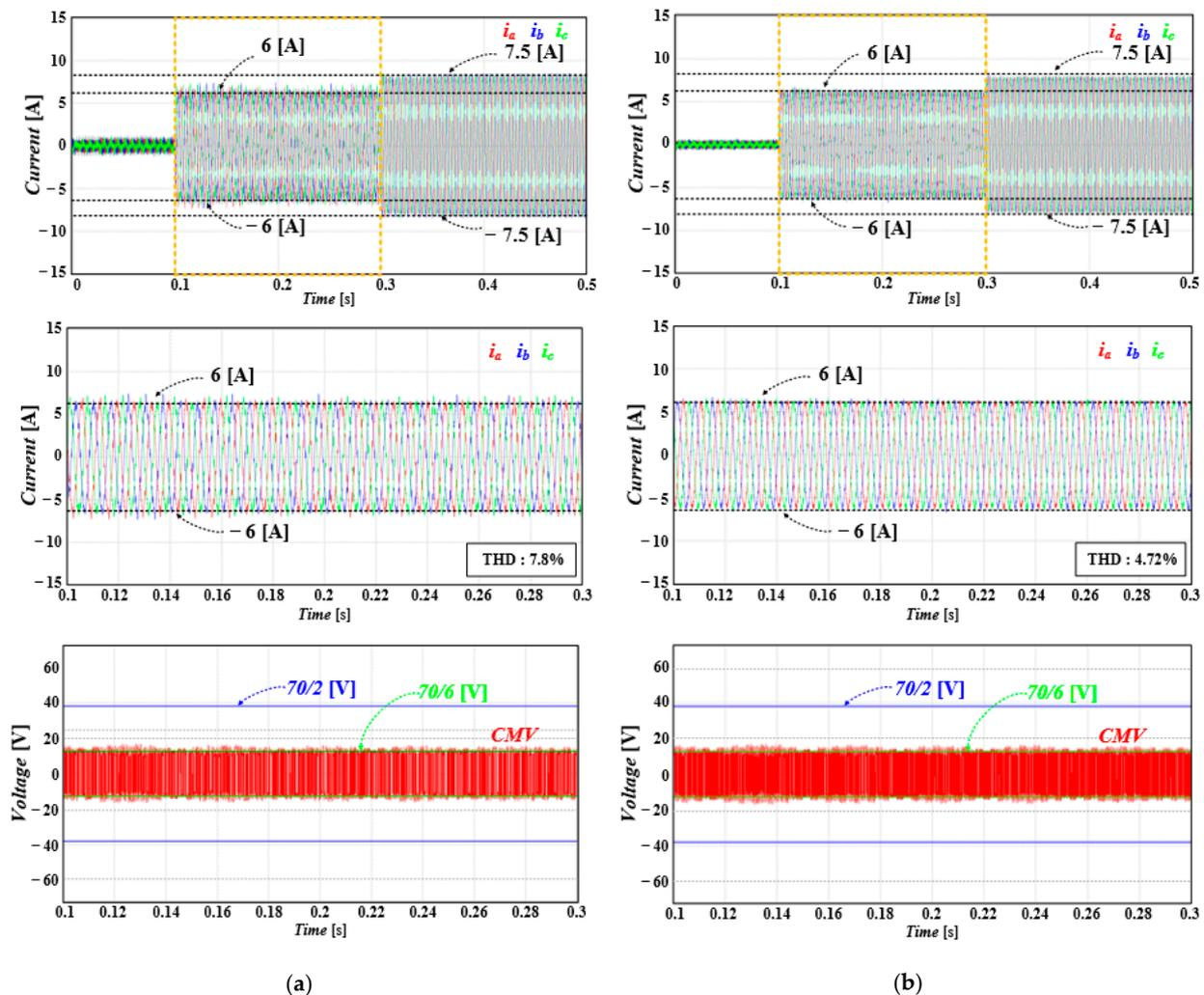
**Figure 12.** Simulation results of FCS-MPC using only non-ZVVs and considering the dead time interval: (a) simulation results with a sampling frequency of 10 kHz and (b) simulation results with a sampling frequency of 20 kHz.
