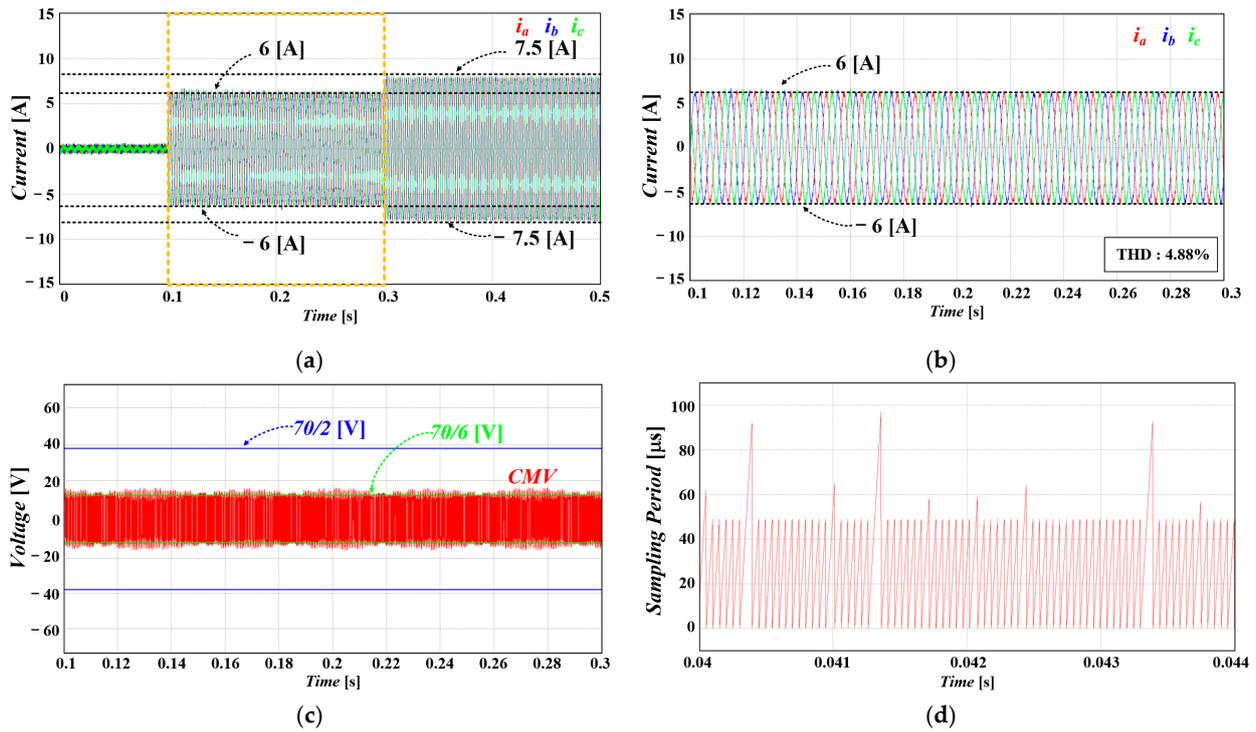
Figure 13. Simulation results of FCS-MPC for CMV reduction with the proposed variable sampling frequency: (a)  $i_a$ ,  $i_b$ , and  $i_c$ ; (b) magnified waveforms of (a); (c) CMV; and (d) sampling period.
