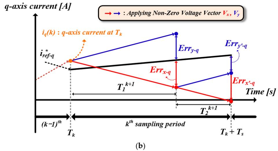
Figure 4. FCS-MPC for reducing current ripple: (a) applying a high sampling frequency and (b) synthesizing two non-ZVVs within one sampling interval. \* expresses the reference value.
