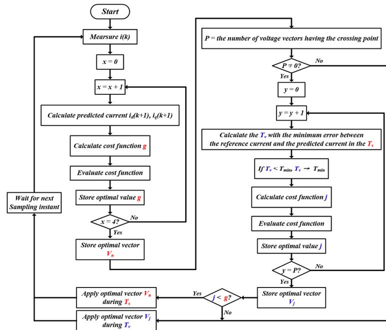
Figure 9. FCS-MPC algorithm for CMV reduction with proposed variable sampling period.
