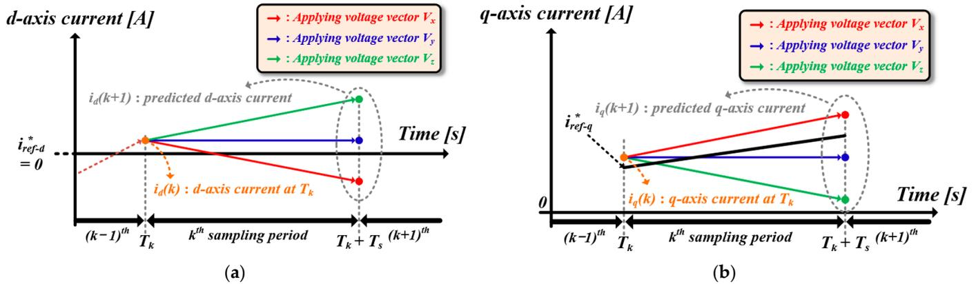
Figure 2. Predicted d-axis and q-axis currents by VVs: (a) predicted d-axis currents and (b) predicted q-axis currents. \* expresses the reference value.
