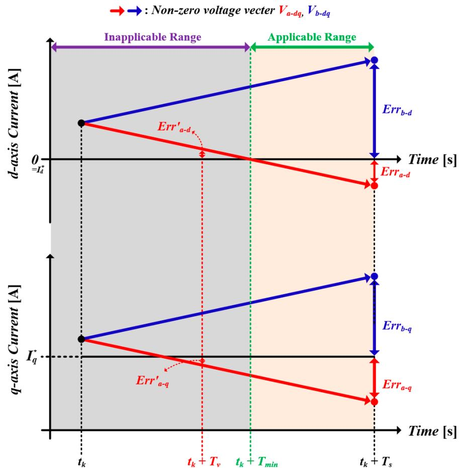
Figure 8. Interval in which variable sampling can be applied.
