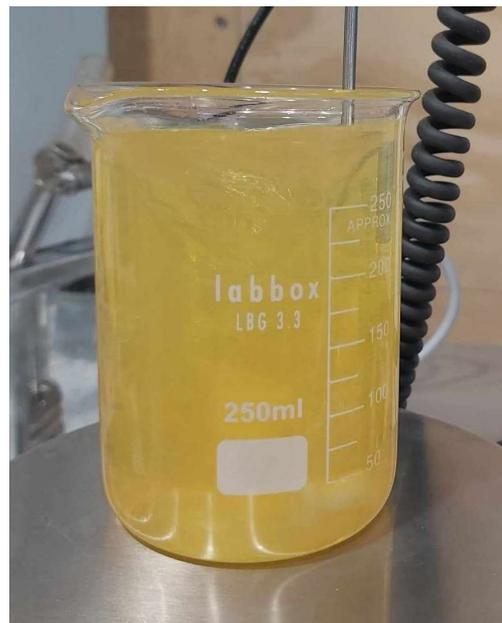
**Figure 4.** The 8% Water-in-Diesel Emulsion (WiDE) at  $T = 40\text{ }^{\circ}\text{C}$ .
