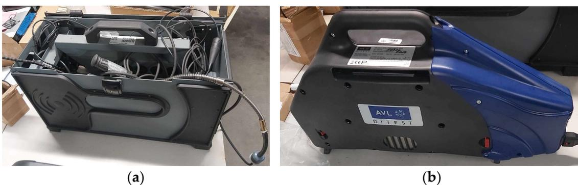
**Figure 10.** (a) AVL DiTest gas 1000 model 2301 5-gas analyzer; (b) AVL DiSmoke 480 opacimeter.
