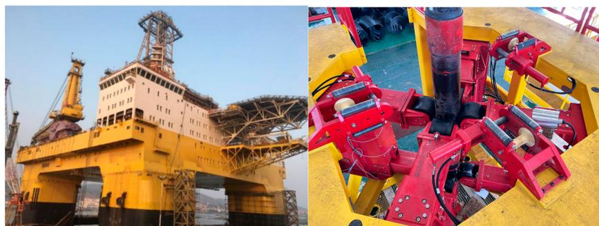
**Figure 13.** Operations vessel “Blue Whale I” and BOP trolley.
