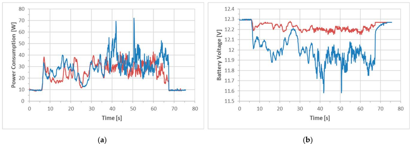
**Figure 15.** Comparative energy diagrams between lead–acid (blue color) and LiPo (red color) batteries for the steps with cargo scenario in rough field terrain: (a) power consumption in Watt; (b) battery voltage in Volt.**Table 8.** Power consumption comparison between lead–acid and Li-Po batteries in the steps with cargo in the rough field terrain scenario.
