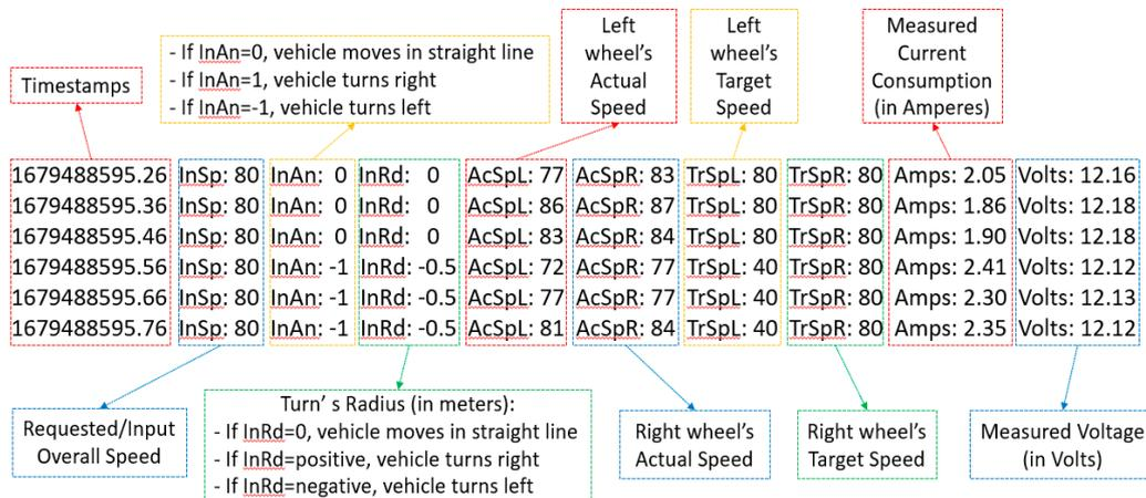
Figure 5. A typical log file of the electric robot.
