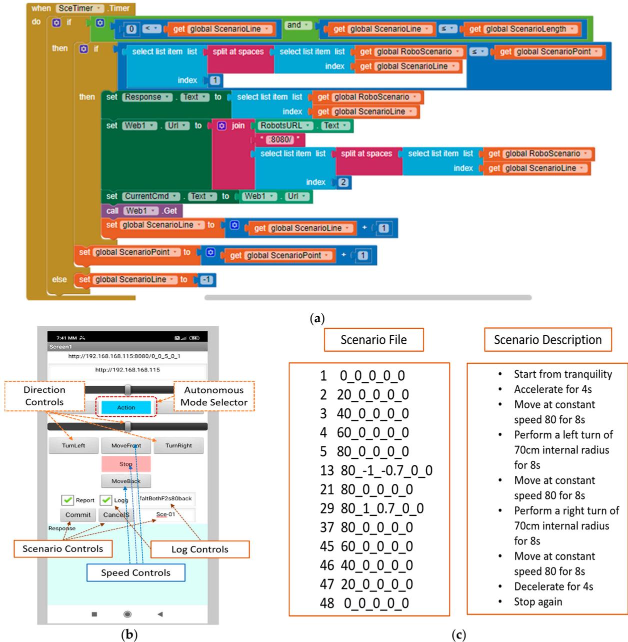
**Figure 4.** (a) An instance of the corresponding code blocks; (b) the application’s interface; (c) indicative scenario file.
