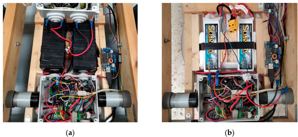
**Figure 8.** Different power source settings, including: (a) sealed lead–acid batteries; (b) Li-Po batteries.
