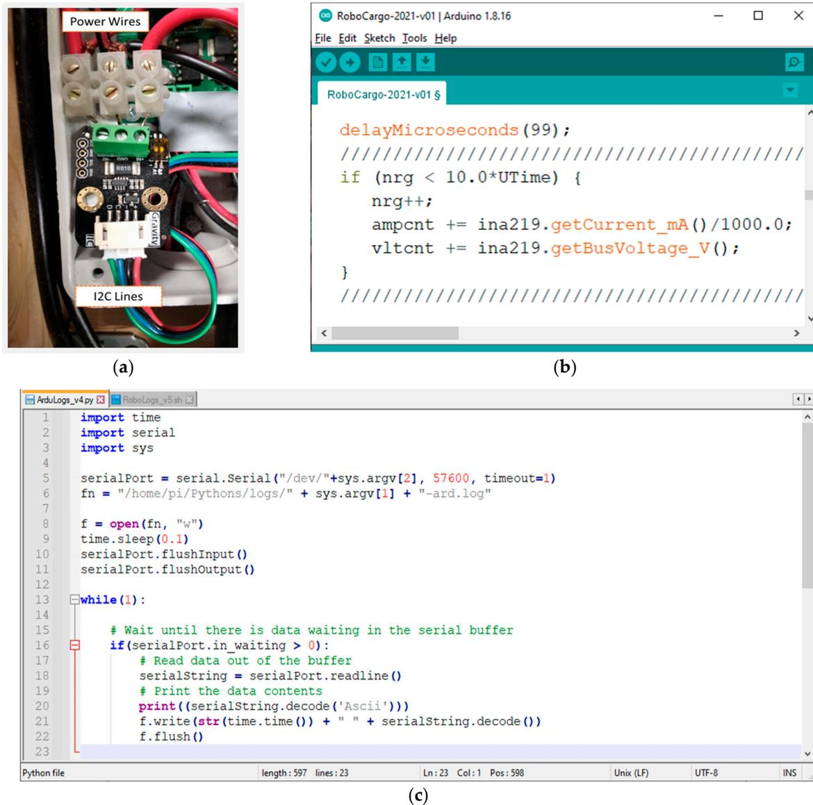
**Figure 3.** (a) The INA219 measuring circuit as incorporated into the robot; (b) a characteristic microcontroller code part for extracting current and voltage measurements; (c) a Python script for handling the microcontroller-originated logging information.
