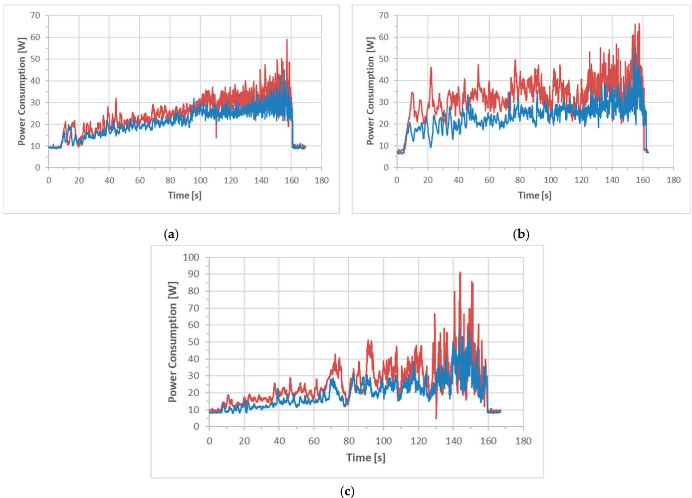
**Figure 9.** Power consumption with cargo (red color) and without cargo (blue color) for the “ramp” scenario in the following: (a) asphalt terrain; (b) grass terrain; (c) rough field terrain.
