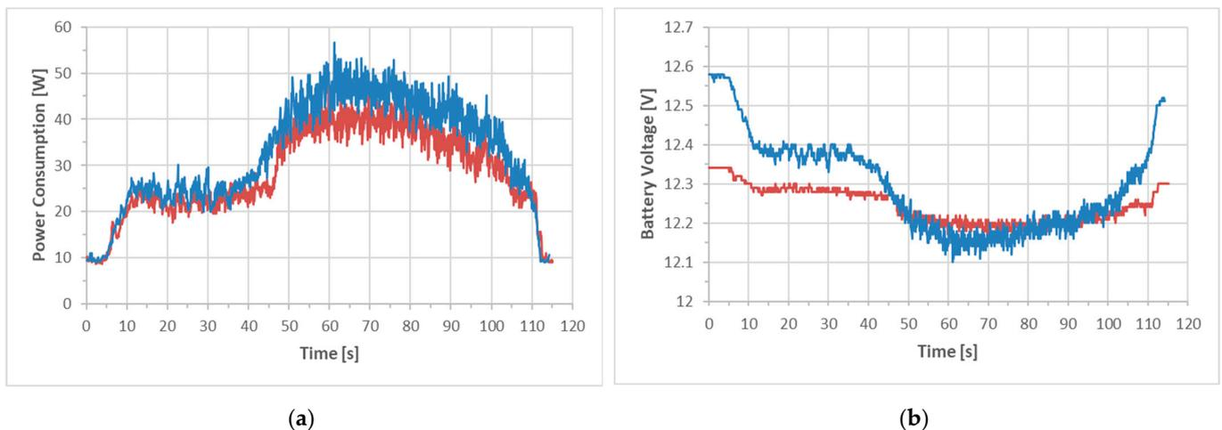
**Figure 16.** Comparative energy diagrams between lead–acid (blue color) and LiPo (red color) batteries during the robot’s straight-line movement in 10% inclined asphalt terrain with 80% of its maximum speed and without cargo: (a) power consumption in Watt; (b) battery voltage in Volt.
