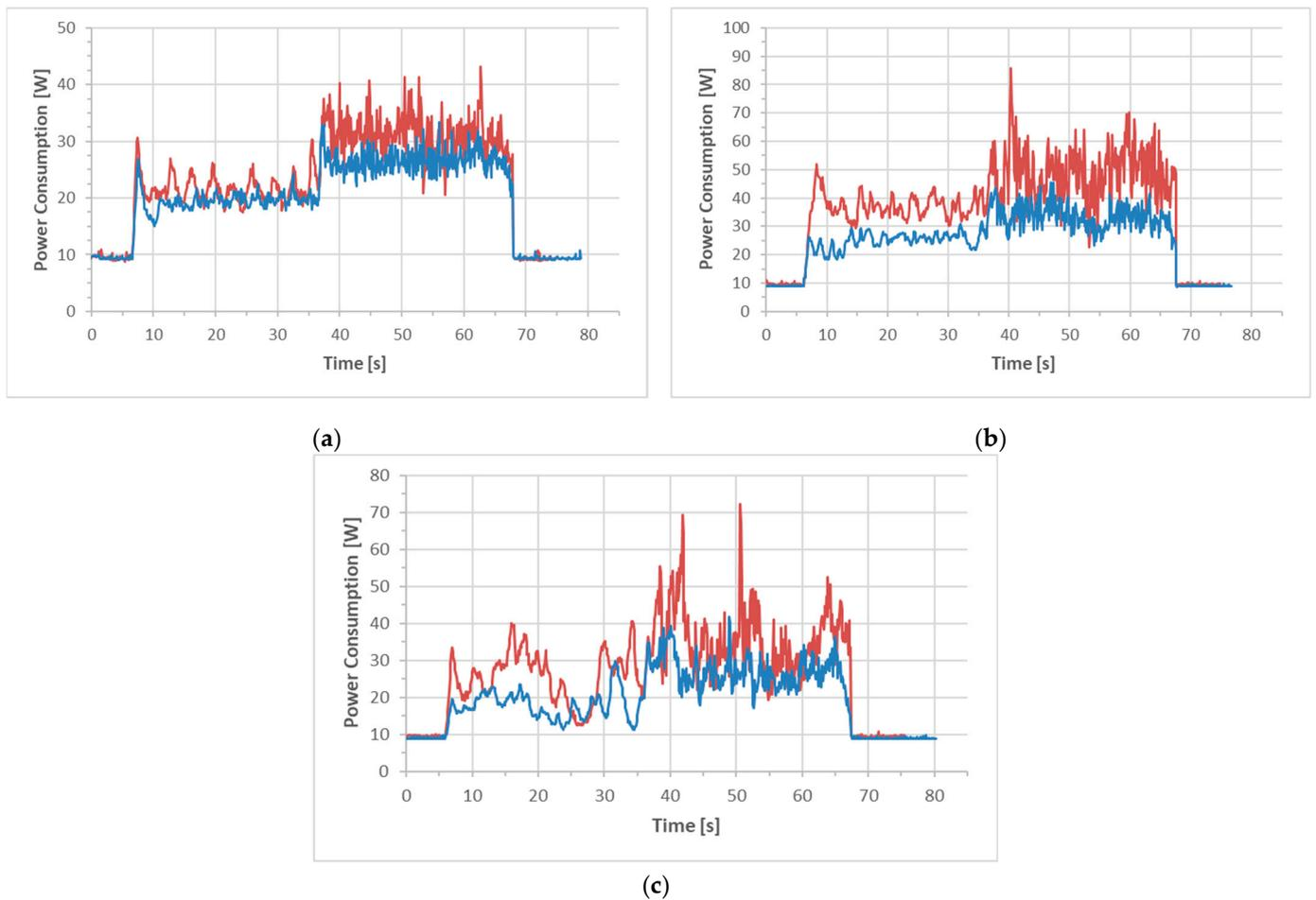
**Figure 10.** Power consumption with (red color) and without (blue color) cargo for the steps scenarios, using lead–acid batteries, on the following: (a) asphalt terrain; (b) grass terrain; (c) rough field terrain.
