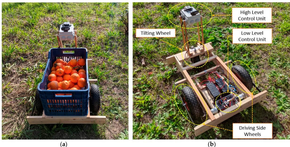
**Figure 1.** The electric cargo robot used in the experiments. (a) Containing a typical cargo of oranges; (b) exhibiting its separate functioning modules.
