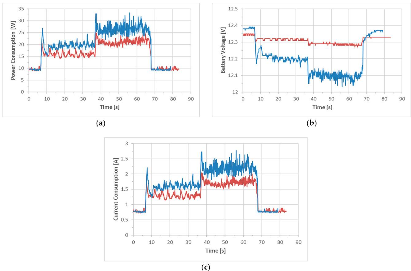
**Figure 13.** Comparative energy diagrams between sealed lead–acid (blue color) and LiPo (red color) batteries for the steps without cargo scenario in asphalt terrain: (a) power consumption in Watt; (b) battery voltage in Volt; (c) current consumption in Ampere.
