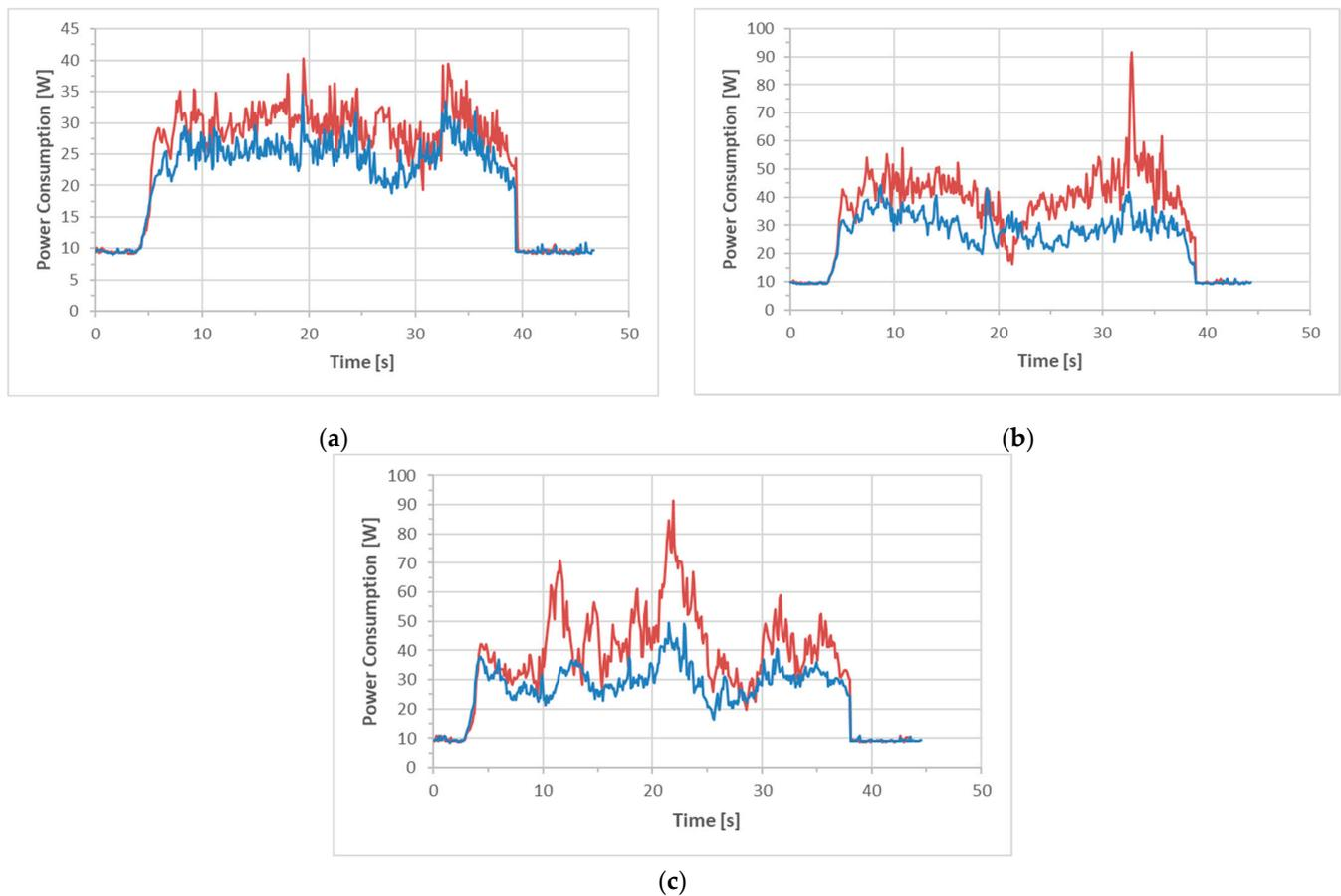
**Figure 11.** Power consumption with (red color) and without (blue color) cargo for the U-turn scenario on the following: (a) asphalt terrain; (b) grass terrain; (c) rough field terrain.
