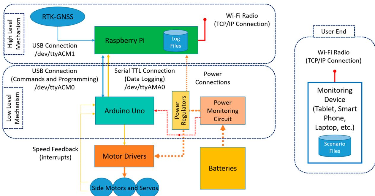
**Figure 2.** Overview of the main control and monitoring mechanism of the electric robotic vehicle utilized in the experiments.
