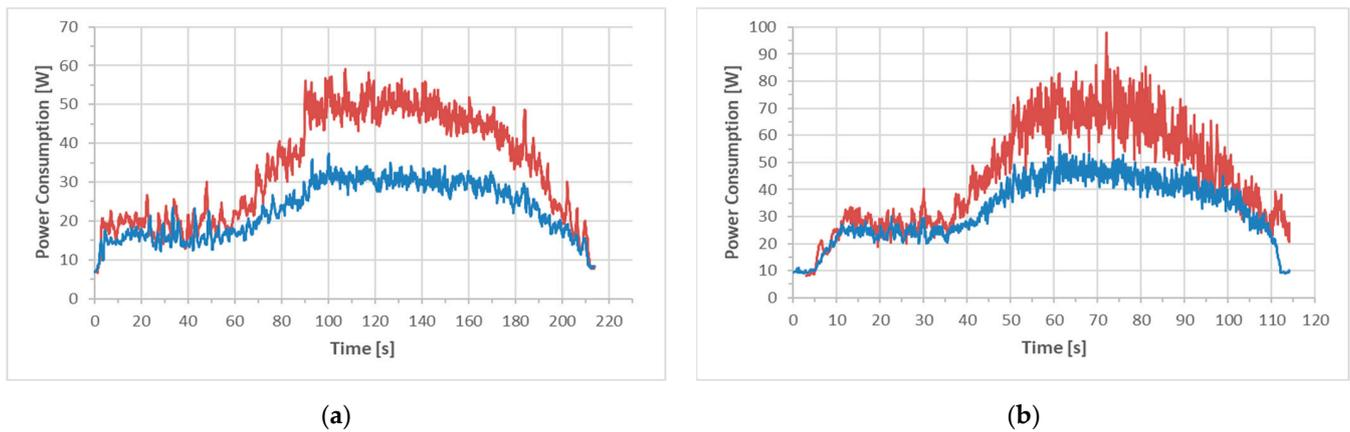
**Figure 12.** Power consumption during the robot's straight-line motion in 10% inclined asphalt terrain with constant speed: (a) 40% of the robot's maximum speed; (b) 80% of the robot's maximum speed. Blue color indicates without cargo scenario and red color with cargo scenario.
