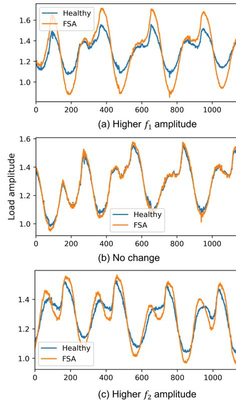
**Figure 6.** Examples of the results of FSA on LSTM time-series inputs.
