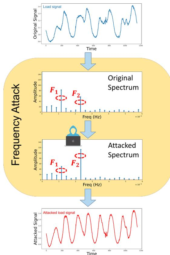
**Figure 1.** The schematic of the proposed FSA operation.
