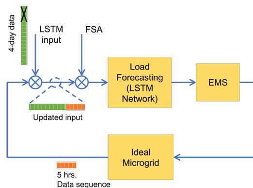
**Figure 8.** The schematic of a microgrid EMS under Frequency Spectrum Attack.
