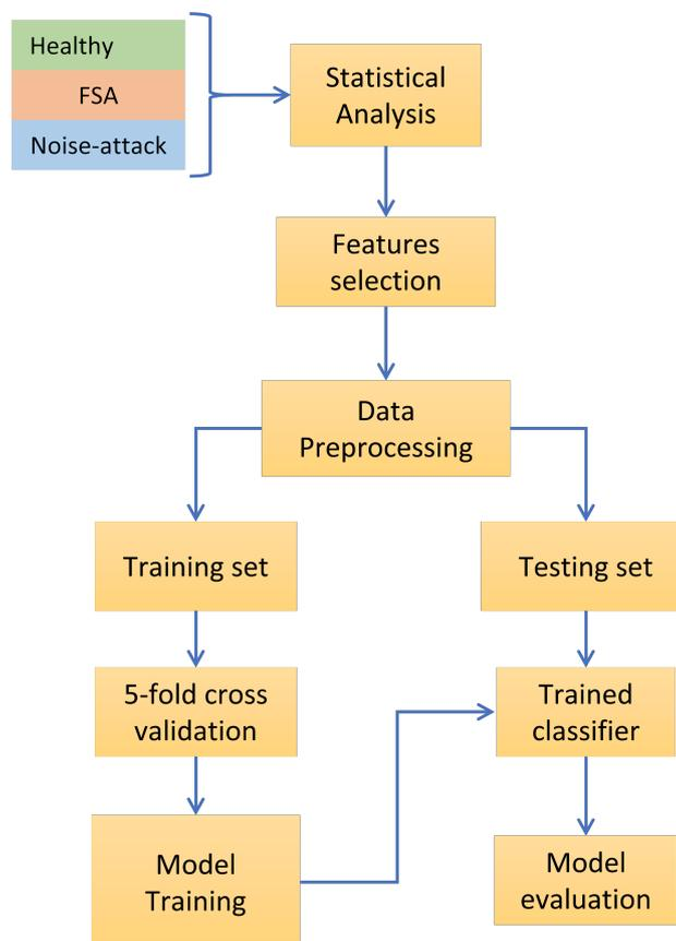
**Figure 16.** The block diagram of the machine-learning-based attack detection.
