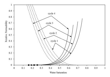
**Figure 3.** The relative permeability curves for water (shown by dotted lines) and CO<sub>2</sub> (represented by solid lines) are utilised in the four WAG injection cycles. The top curve corresponds to CO<sub>2</sub> injection, while the bottom curve corresponds to water injection.
