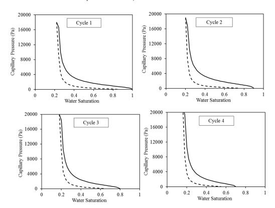
**Figure 4.** Capillary pressure curves employed for the four cycles of WAG injection. The solid lines reflect the CO<sub>2</sub> injection, while the dashed lines illustrate the water injection.
