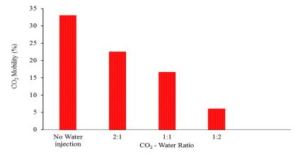
Figure 6. The proportion of free  $CO_2$  relative to the total amount of injected  $CO_2$ , expressed as a function of the  $CO_2$ -water ratio at the completion of the  $CO_2$  storage period. The  $CO_2$ -water ratio strategy of 1:2 is considered to be the most optimal.
