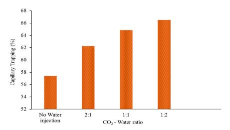
Figure 7. The ratio of  $CO_2$  that is trapped in capillary compared to the total amount of  $CO_2$  injected, represented as a function of the ratio of  $CO_2$  to water at the end of the  $CO_2$  storage period. The 1:2  $CO_2$ -water ratio is regarded as the most optimal.
