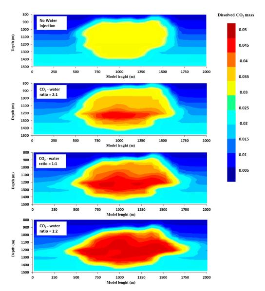
**Figure 9.** Dissolved  $CO_2$  mass fraction as a function of the  $CO_2$ -water ratio, at the end of the  $CO_2$  storage time.
