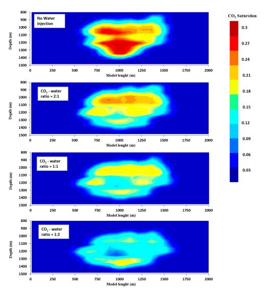
**Figure 5.** Two-dimensional cross-sectional viewpoints of the reservoir displaying the  $CO_2$  plume with the saturation of supercritical  $CO_2$  for the different  $CO_2$ -water ratio scenarios at the end of the  $CO_2$  storage period.
