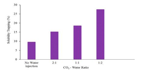
Figure 8. The ratio of  $CO_2$  that is trapped in solubility trapping compared to the total amount of  $CO_2$  injected, represented as a function of the ratio of  $CO_2$  to water at the end of the  $CO_2$  storage period. The 1:2  $CO_2$ -water ratio is regarded as the most optimal.
