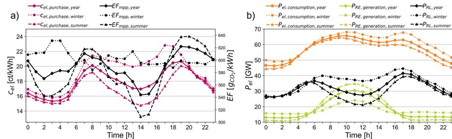
**Figure 3.** (a) Hourly average electricity costs and hourly average EF. (b) Composition of the hourly average RL.
