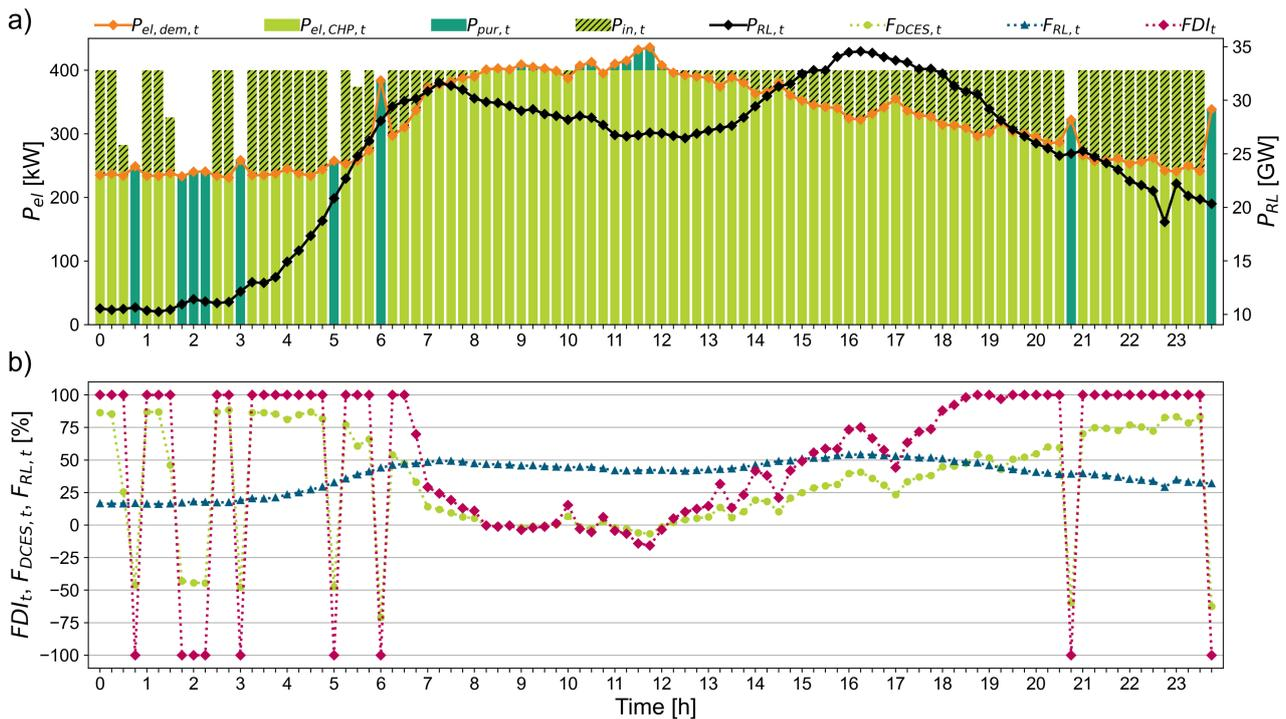
**Figure 4.** (a) The DCES electrical key figures in quarter-hourly resolution of the *opt* concept in the *EF* tariff and the absolute RL for an exemplary day in winter. (b) The corresponding  $F_{DCES,t}$  and  $F_{RL,t}$  for every time step result in the  $FDI_t$ .
