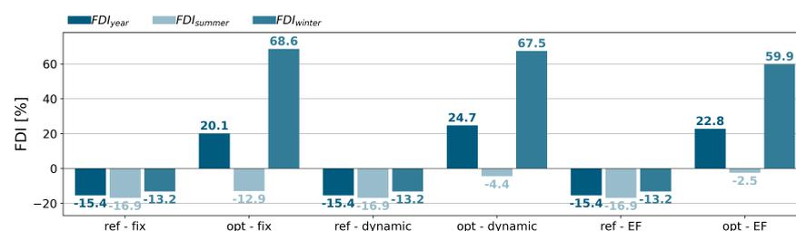
**Figure 5.** The FDI of relevant QPs for two concepts in three tariff scenarios. The  $\overline{FDI}$  is presented for the QP of one year, the summer time, and the winter time.
