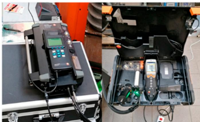
**Figure 4.** Flue gas analyzers used in the tests. On the left: Testo 350 S; on the right: Testo 380 and Testo 330-2 LL.
