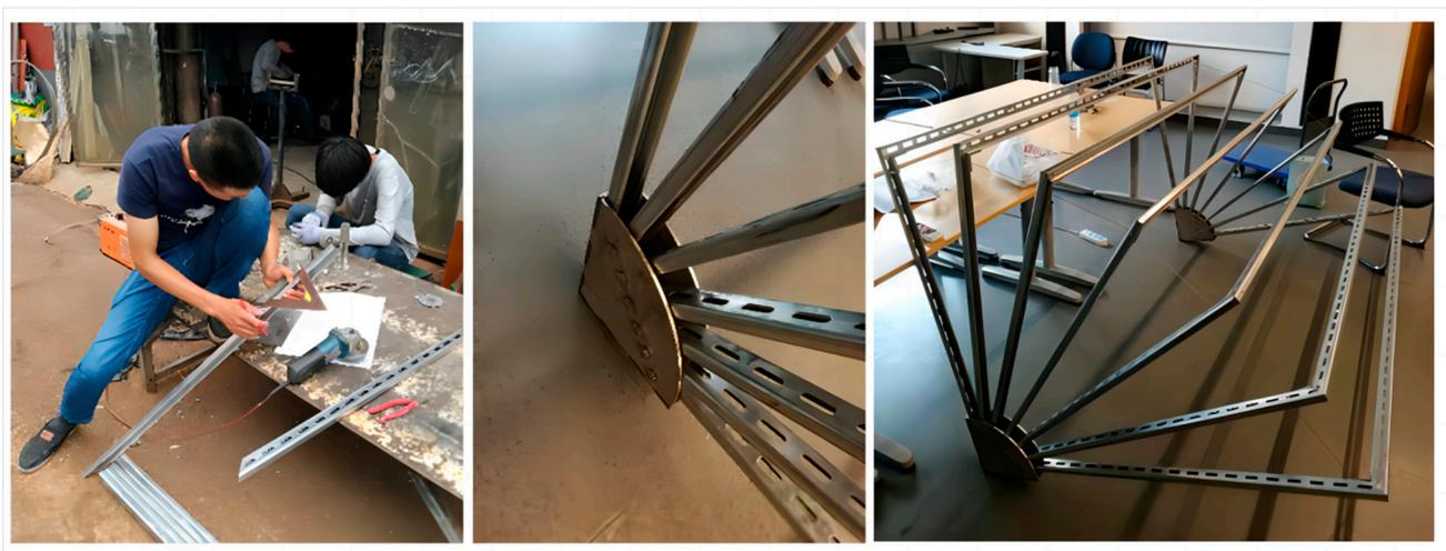
**Figure 4.** Production of opening-closing skeleton.
