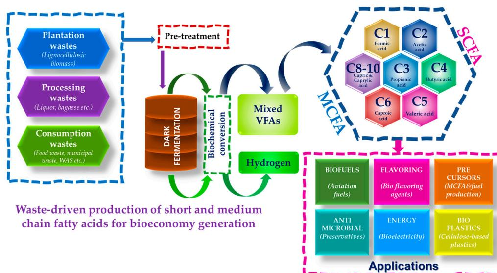
**Figure 2.** Fermentative organic waste bioconversion into biobased products.
