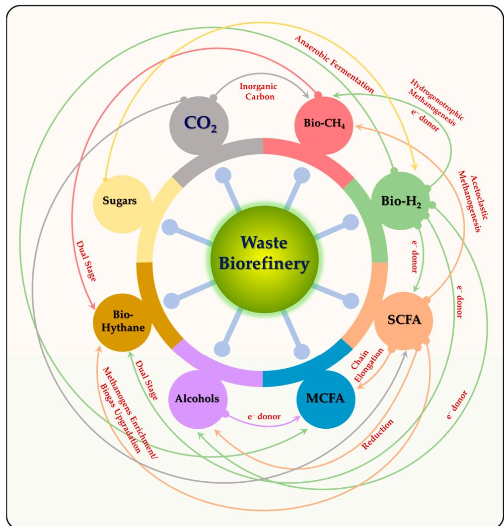
Figure 4. Waste biorefinery model integrated with multiple processes.
