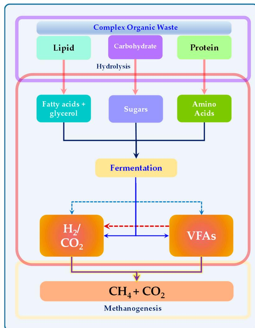
**Figure 1.** Schematic representation of anaerobic fermentation stages.
