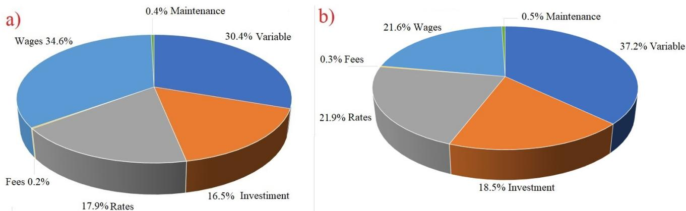
**Figure 3.** Cost composition of hydrogen production plants. (a) one electrolysis kit, (b) five electrolysis kit.
