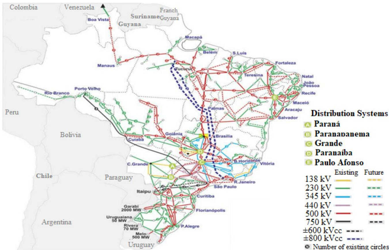
Figure 1. Scheme of smart grid of the Brazilian electrical system [4,13].
