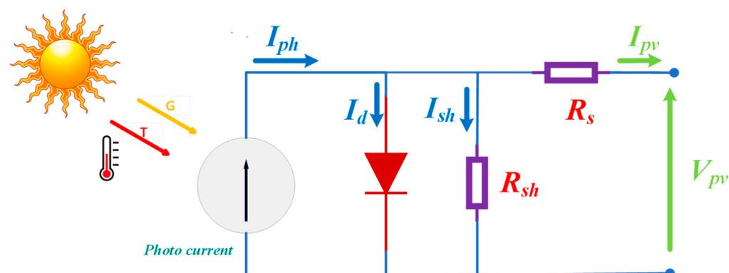
Figure 3. ODM of PV cell.
