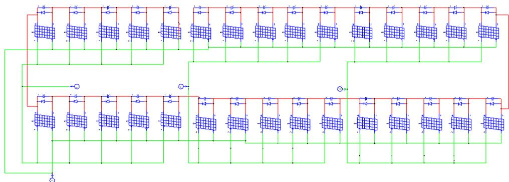
Figure 8. PV array and DC–DC boost converter circuits employed in Psim environment.
