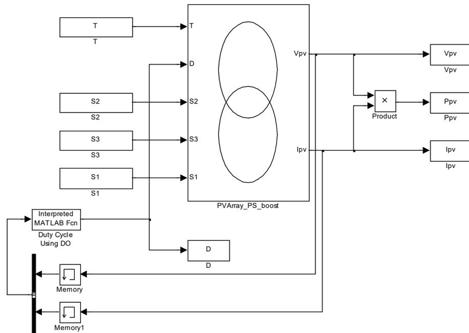
Figure 7. Implemented Matlab/Simulink model for MPPT algorithms.
