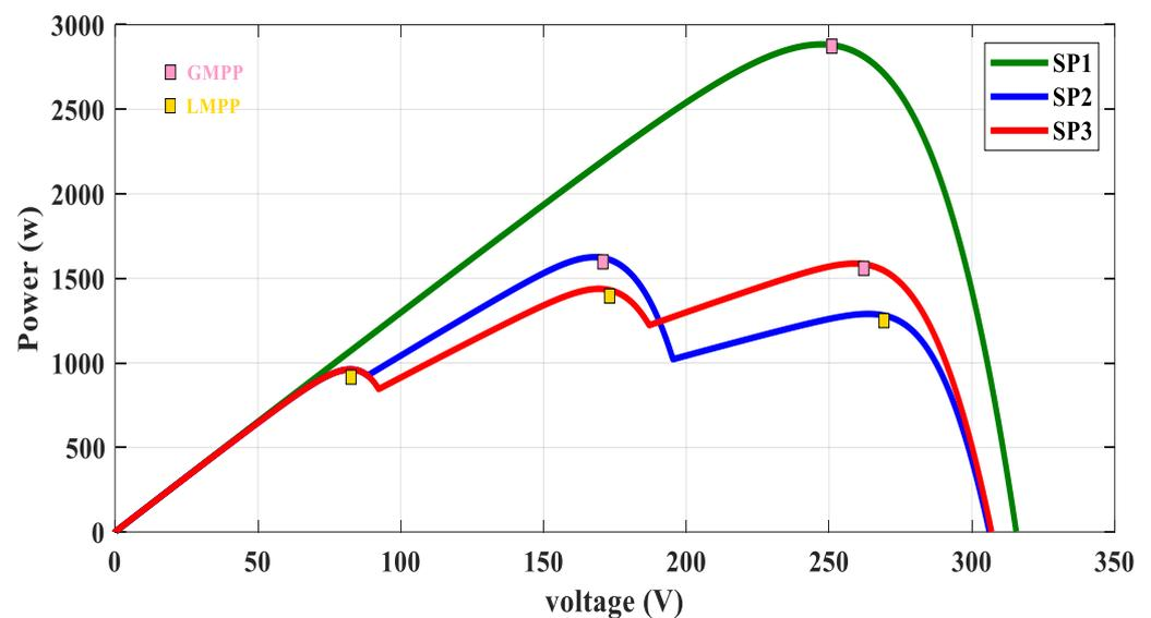
**Figure 9.** Shading patterns.
