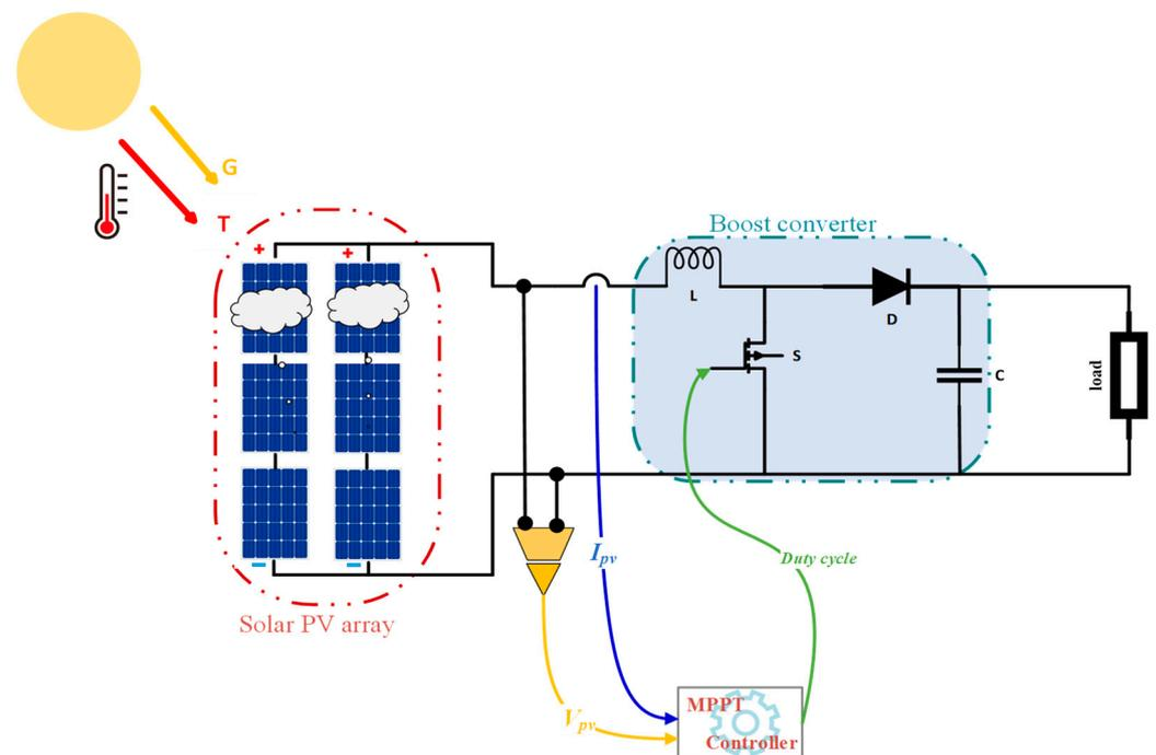
**Figure 1.** Illustration of PV System with Boost Converter for MPPT.
