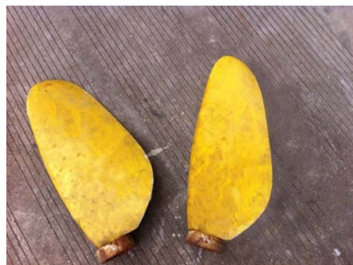
Figure 12. Comparison of two blades with different solidity.
