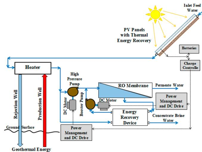
Figure 1. Simplified schematics of the proposed RO desalination cycle.
