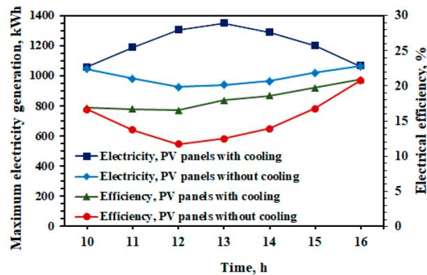
Figure 5. Variation of electricity generation and electrical efficiency from PV panels with and without the thermal recovery system.
