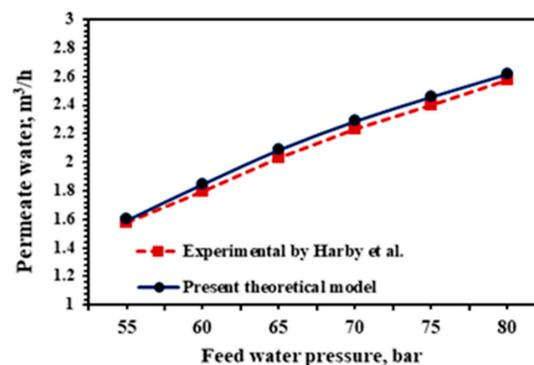
Figure 3. Model validation of the RO desalination unit [34].
