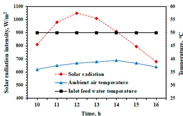
**Figure 4.** Variations of sunrays, ambient temperature, and feed water temperature.
