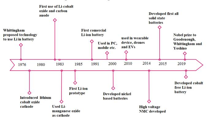
Figure 1. Major breakthroughs in LBs and its related technologies.
