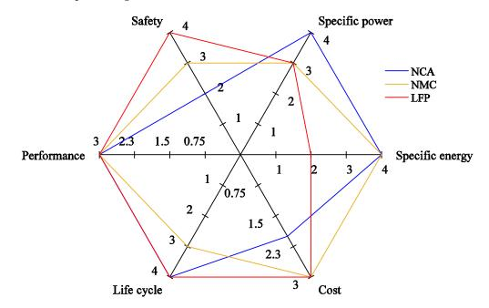
Figure 4. Performance parameters of various battery chemistries.
