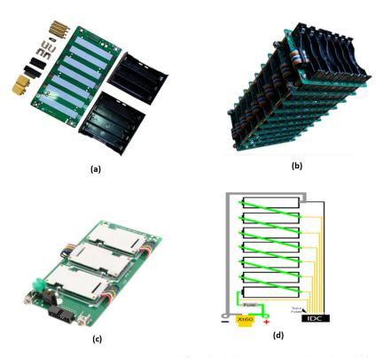
Figure 12. Open-source, Do-it-yourself modular battery storage kit: (a) exploded view; (b) assembled and stacked; (c) battery management module; (d) simplified circuit representation of the battery module [128].
