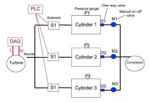
Figure 14. Main components of the modular low-pressure micro-CAES [146].
