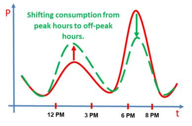
Figure 9. Load shifting using demand-side energy flexibility [51].
