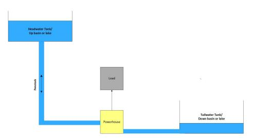
Figure 6. Working principle of pumped hydroelectric storage stations.
