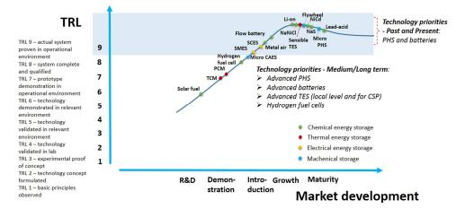
**Figure 11.** Overview of the maturity of energy storage technologies (Thermo-Chemical Materials (TCMs), phase change materials (PCMs), superconducting magnetic energy storage (SMES), super capacitor energy storage (SCES), sodium nickel chloride (NaNiCl) batteries, thermal energy storage (TES), nickel cadmium (NiCd) batteries, sodium sulphur (NaS) batteries, and pumped hydro storage (PHS)) as of 2017 with technology readiness level (TRL) on the y-axis and market development on the x-axis [120].
