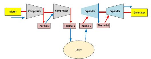
Figure 13. Working principle of compressed air energy storage systems [142].
