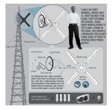
Figure 3. William Kamkwamba's windmill design and components [24].
