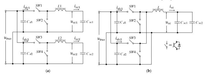
**Figure 15.** Parallel topology *DC/DC* conversion with single-phase conversion method: (**a**) option 1; (**b**) option 2.
