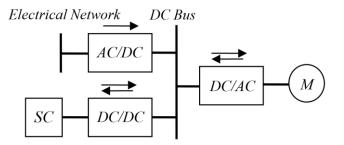
Figure 10. A combined crane electric drive system with mains supply as the main energy source.
