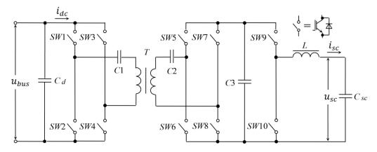
Figure 17. Full bridge resonant DC/DC converter topologies.
