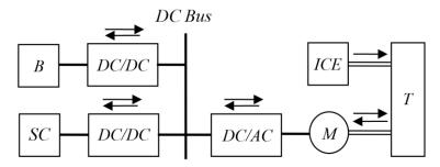
Figure 1. Combined vehicle system with *ICE* as the main energy source.
