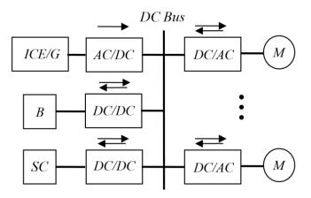
Figure 2. Combined 4WD vehicle system with *ICE/G* as main power source.
