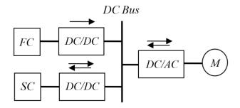
Figure 7. Combined vehicle system with *FC* as the main power source.
