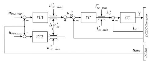
Figure 21. Three-circuit ACS of a supercapacitor energy storage.
