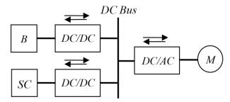
Figure 6. Combined vehicle system with a controlled battery as the main power source.
