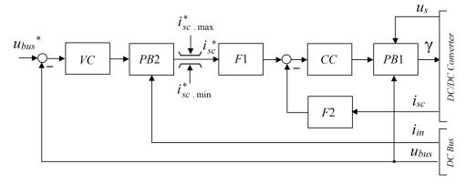
Figure 20. Generalised two-circuit ACS of supercapacitor energy storage.
