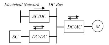
**Figure 11.** A combined lift electric drive system with a power supply network as the main energy source and a backup source *FC*.
