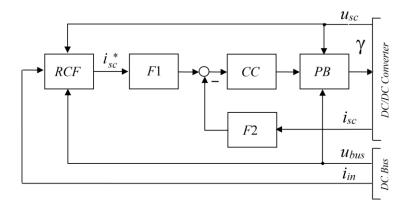
Figure 19. Generalised single-circuit ACS of a supercapacitor energy storage.
