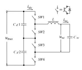
Figure 14. Three-level topology of DC/DC converter.
