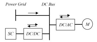
Figure 9. Combined traction drive system with *DC* mains as the main power source.
