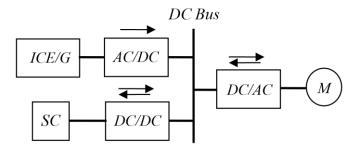
Figure 4. Combined truck drive system with ICE/G as main power source.
