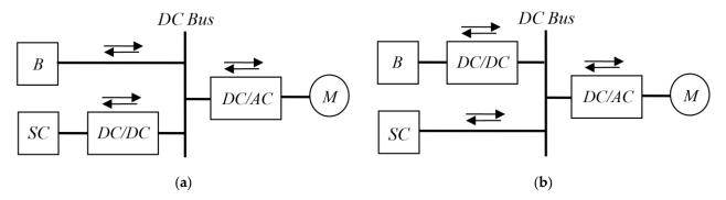
**Figure 5.** Combined vehicle system with a battery as the main power source: (**a**) first topology; (**b**) second topology.
