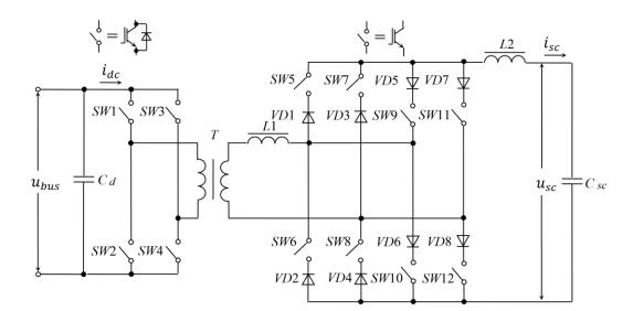
Figure 18. ZVT/ZCS converter topologies.
