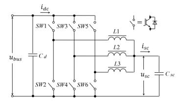
Figure 16. Topology of a three-phase DC/DC interleaved converter.
