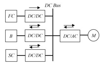
**Figure 8.** Combined vehicle system with *FC* as the main energy source and controllable auxiliary sources *B* and *SC*.
