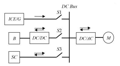
Figure 3. Combined vehicle system with ICE/G as main power source.
