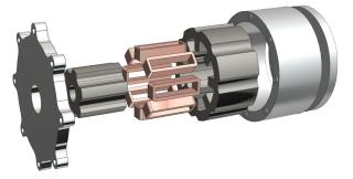
**Figure 25.** Exploded view of Design I with improved bolt and flange mounts and with stator back iron notches.
